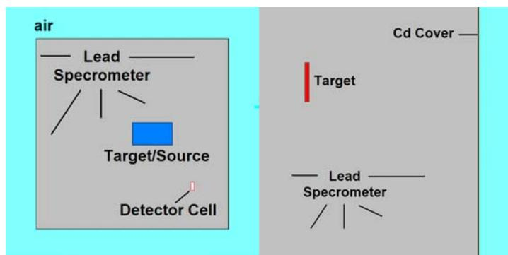
*Cross sections of the UNLV benchmark of the LANL lead SDS taken from MXNPX models. (left) The overall geometry, (right) A close-up of a cross section of the thin target. The response to neutrons of various energies (time constants) is influenced by the position and isotopic composition of the detector.*
