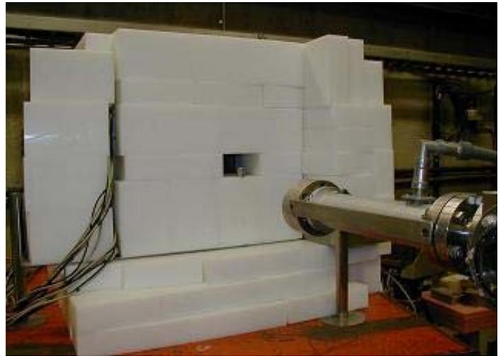
*View of detector system aligned with accelerator vacuum tube and window. The beam height had not been adjusted in this photograph. The AmBe source can be seen in the opening in the polyethylene bricks of the NMDS.*
