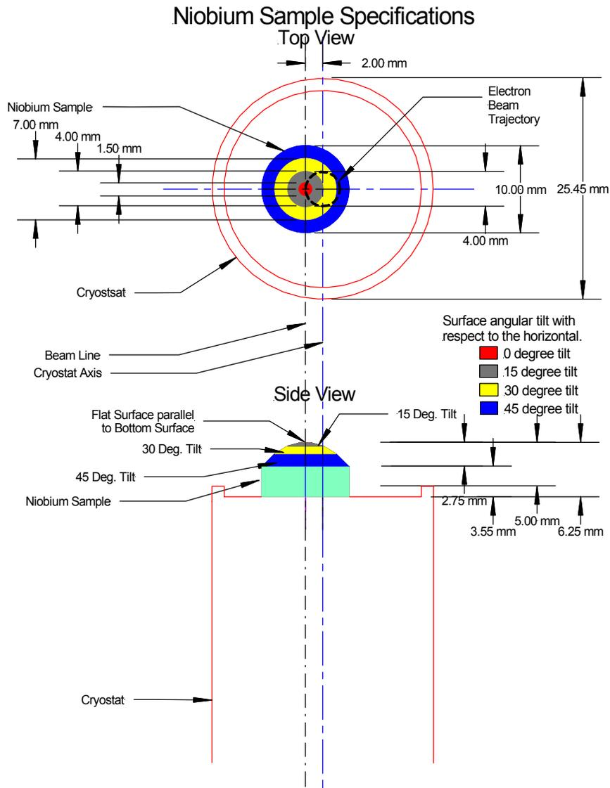
**Fig. 4. Specially designed sample on cryostat mounted on rotatable axis stage (not shown). The cryostat axis is off center of the axis of the electron beam. The top view maps out the position of the electron beam (dashed black line) on the sample under test.**
