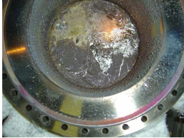
Fig. 3. Slag accumulated on the surface of LBE after 300-hour operation.
