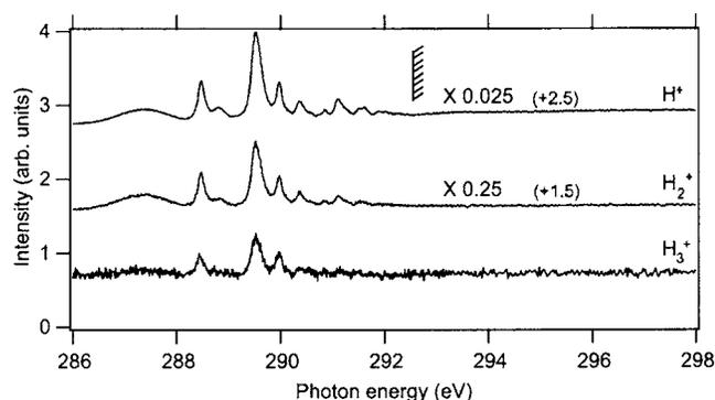
FIG. 13. Partial ion yields of the H<sup>+</sup>, H<sub>2</sub><sup>+</sup>, and H<sub>3</sub><sup>+</sup> fragments in the region of the C1s ionization threshold. Scaling factors and offsets on the vertical axis are shown.
