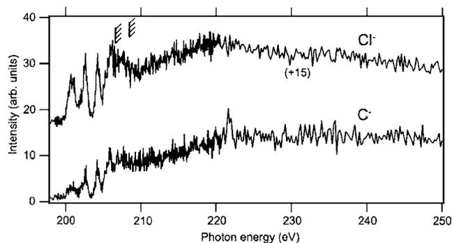
FIG. 9. Partial ion yields of the two detectable anions,  $^{35}Cl^-$  and  $C^-$ , in the region of the  $Cl2p$  ionization thresholds. For clarity an offset is used on the vertical axis for  $Cl^-$ .
