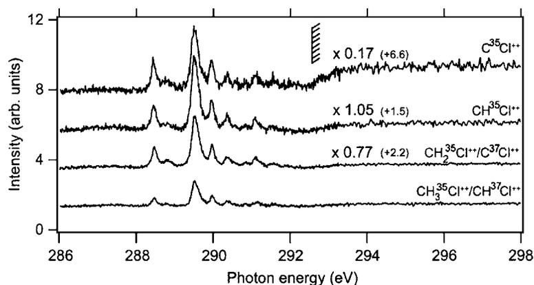
FIG. 12. Partial ion yields of the CH<sub>*i*</sub>Cl<sup>*i*+</sup> fragments (*i*=0–3) around the C1s ionization threshold. Spectra are normalized to the intensity of the first peak (C1s → 8a<sub>1</sub>). Scaling factors and offsets on the vertical axis are shown.
