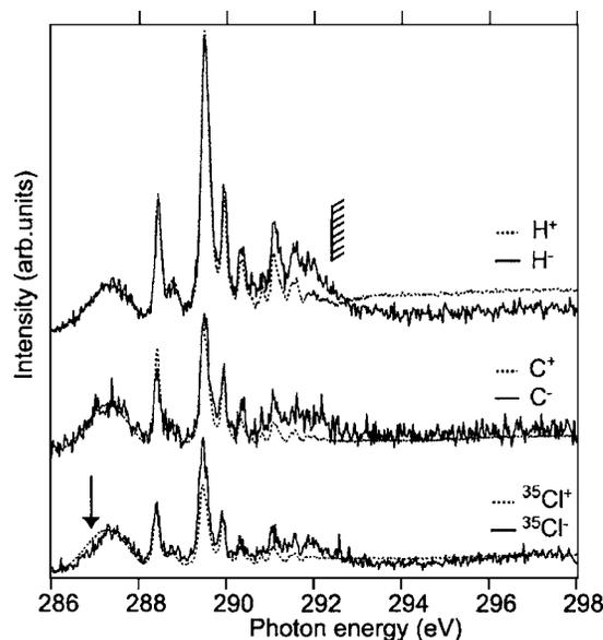
FIG. 14. Partial ion yields of the detectable anions C<sup>-</sup>, <sup>35</sup>Cl<sup>-</sup>, and H<sup>-</sup> fragments around the C1s ionization threshold. These spectra are compared to partial ion yields of C<sup>+</sup>, <sup>35</sup>Cl<sup>+</sup>, and H<sup>+</sup> normalized to the intensity of the C1s → 8a<sub>1</sub> resonance and calibrated in energy at the first Rydberg component. As described in the text, the arrow indicates the zone corresponding to shorter C–Cl bond distances.
