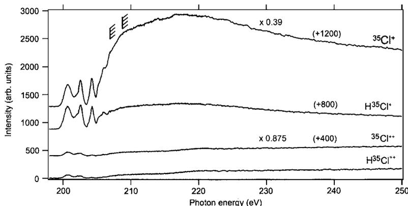
FIG. 8. Partial ion yields of the  $^{35}Cl^+$ ,  $H^{35}Cl^+$ ,  $^{35}Cl^{++}$ , and  $H^{35}Cl^{++}$  fragments around the  $Cl2p$  ionization thresholds. The spectra are normalized to the intensity of the  $Cl2p_{3/2} \rightarrow 8a_1$  transition. Scaling factors and offsets on the vertical axis are shown.
