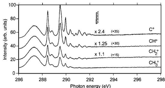
FIG. 11. Partial ion yields of the  $\text{CH}_i^+$  fragments ( $i=0-3$ ) around the  $\text{C}1s$  ionization threshold. Spectra are normalized to the intensity of the first peak ( $\text{C}1s \rightarrow 8a_1$ ). Scaling factors and offsets on the vertical axis are shown.
