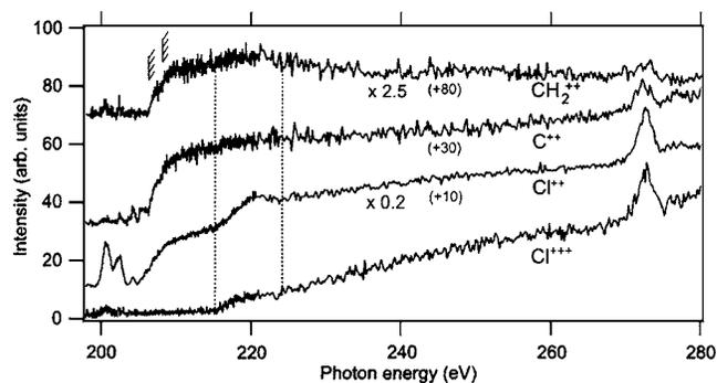
FIG. 6. Comparison of  $^{35}\text{Cl}^{3+}$ ,  $^{35}\text{Cl}^{2+}$ ,  $\text{C}^{2+}$ , and  $\text{CH}_2^{2+}$  ions yields. The dotted lines delimit a zone corresponding to the opening of dissociation pathways involving triply charged species. Scaling factors and offsets on the vertical axis are shown.
