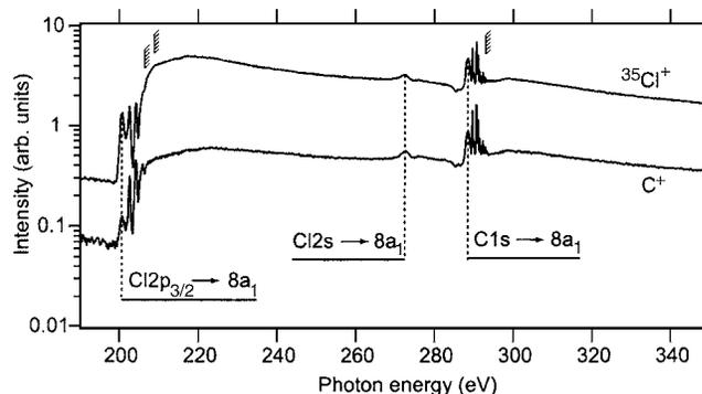
FIG. 1. Partial ion yields of the C<sup>+</sup> and <sup>35</sup>Cl<sup>+</sup> fragments taken over a large photon-energy range including the Cl2*p*, Cl2*s*, and C1*s* edges.
