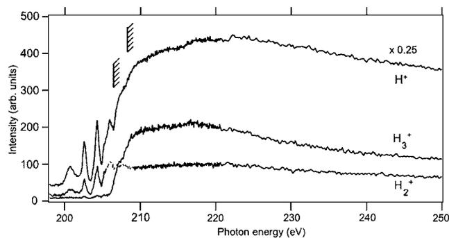
FIG. 7. Partial ion yields of  $H^+$ ,  $H_2^+$ , and  $H_3^+$  fragments in the region of the  $Cl2p$  ionization thresholds. A scaling factor for  $H^+$  is used for clarity.
