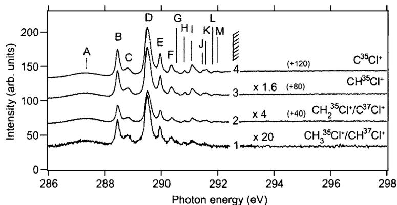
FIG. 10. Partial ion yields of the  $\text{CH}_i\text{Cl}^+$  fragments ( $i=0-3$ ) around the  $\text{C}1s$  ionization threshold. Spectra are normalized to the intensity of the first peak ( $\text{C}1s \rightarrow 8a_1$ ). Scaling factors and offsets on the vertical axis are shown. Labels refer to Table II.
