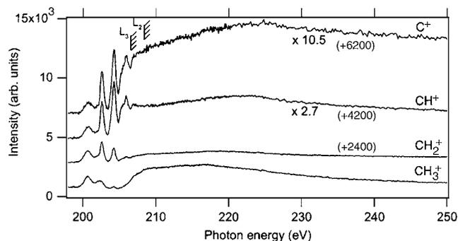
FIG. 3. Partial ion yields of the  $\text{CH}_i^+$  fragments ( $i=0-3$ ) around the  $\text{Cl}2p$  ionization thresholds. Spectra are normalized to the intensity of the first peak ( $\text{Cl}2p_{3/2} \rightarrow 8a_1$ ). Scaling factors and offsets on the vertical axis are shown. Positions of the  $\text{Cl}2p_{3/2}$  and  $\text{Cl}2p_{1/2}$  ionization potentials are indicated by  $L_3$  and  $L_2$ , respectively.
