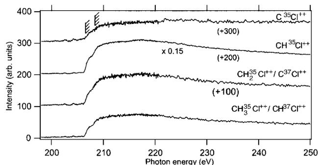
FIG. 4. Partial ion yields of the  $\text{CH}_i\text{Cl}^{i+}$  fragments ( $i=0-3$ ) around the  $\text{Cl}2p$  ionization thresholds. A scaling factor and offsets on the vertical axis are shown.
