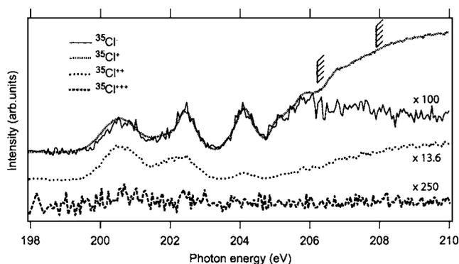
FIG. 5. Qualitative comparison of partial ion yields of the  $^{35}\text{Cl}^-$ ,  $^{35}\text{Cl}^+$ ,  $^{35}\text{Cl}^{2+}$ , and  $^{35}\text{Cl}^{3+}$  fragments below the  $\text{Cl}2p$  ionization thresholds. Scaling factors are used to normalize the spectra to the intensity of the first transition.
