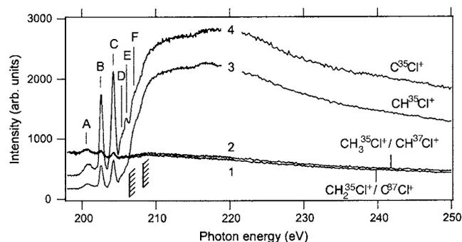
FIG. 2. Partial ion yields of the  $\text{CH}_i\text{Cl}^+$  fragments ( $i=0-3$ ) around the  $\text{Cl}2p$  ionization thresholds. Labels refer to Table I.
