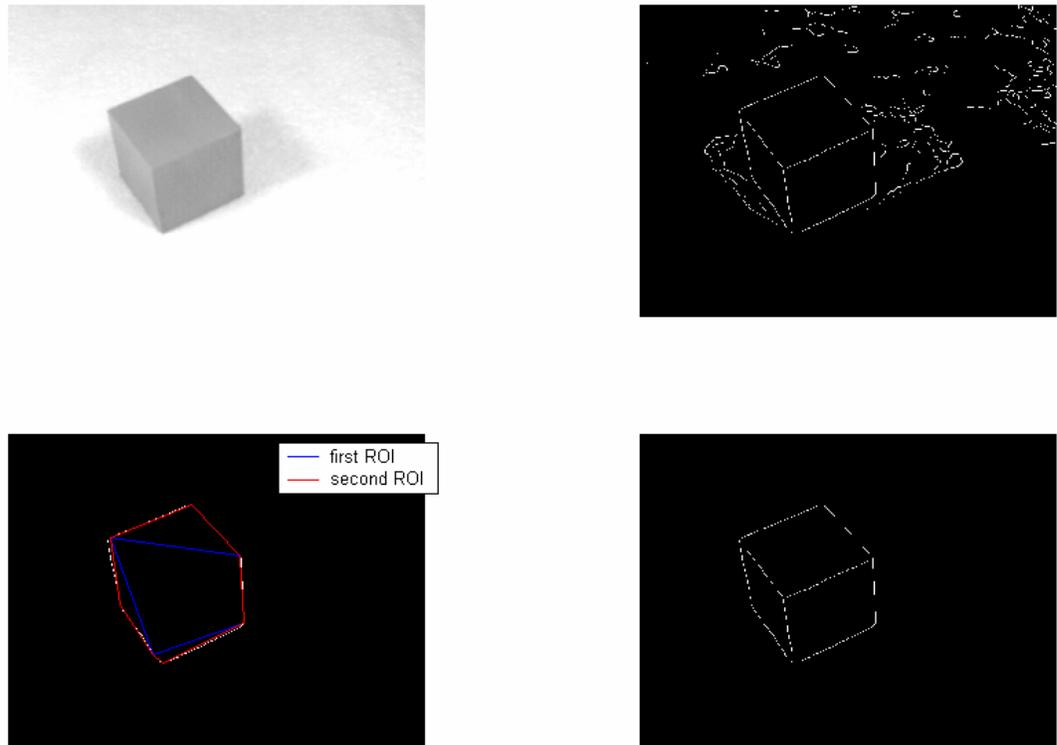
Figure 3.5. Machine Recognition in Matlab. (Top Left: Original Photograph, Top right: Segmented Image containing Noise, Bottom Left: Steps of the Object Identification Process, Bottom Right: Object is correctly identified as a cube.)
