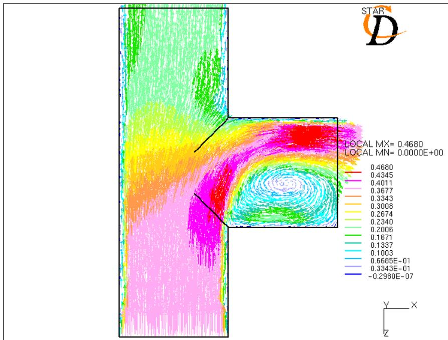
Figure 3.6: Velocity vectors for a side inlet (from bottom inlet) t-joint at  $Re = 200,000$  (turbulent flow)
