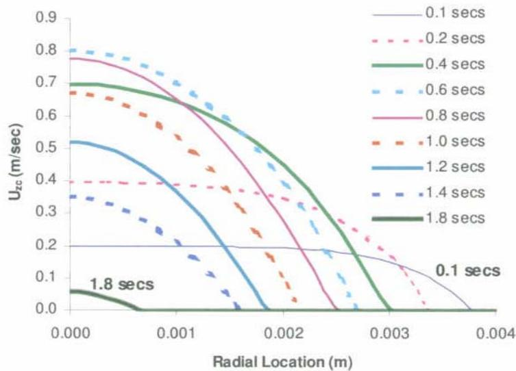
Figure 3.1. Axial velocity profile for constant inlet pressure of 20 kPa (Mold temperature = 400 °C, initial melt temperature = 1500 °C, interfacial heat transfer coefficient = 2,000 W/m<sup>2</sup>-K)
