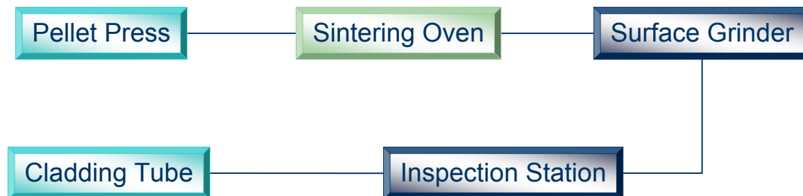
Figure 3.3. Material Flow in Hot Cell.
