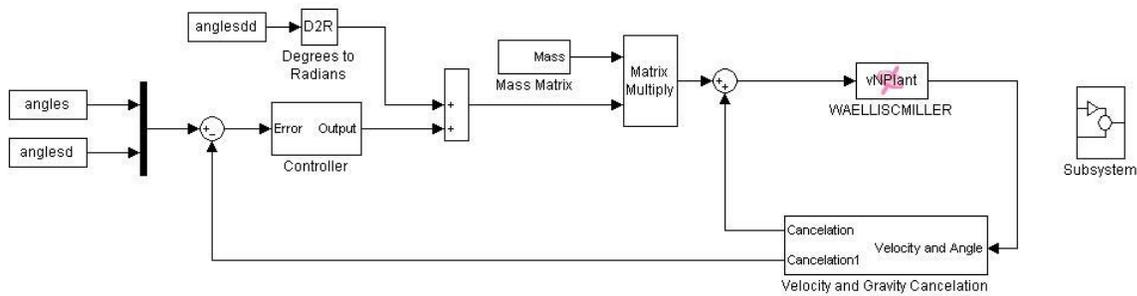
Figure 3.2. Computed Torque method implemented in MATLAB
