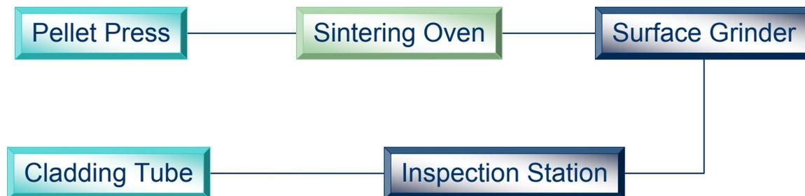
Figure 3.3. Material Flow in Hot Cell.
