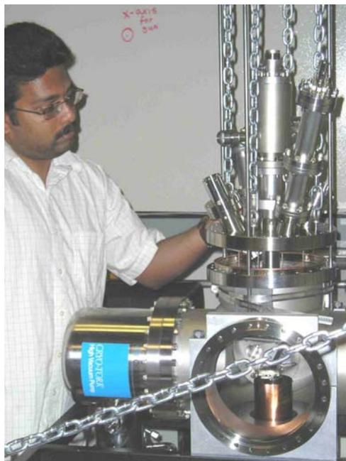
Fig. 2. Anoop George (graduate student) assembling the detector and gun assembly to the vacuum chamber. The electron gun (centered in vertical position on the top flange) and RGA head (offset angle to right of gun) are displayed.
