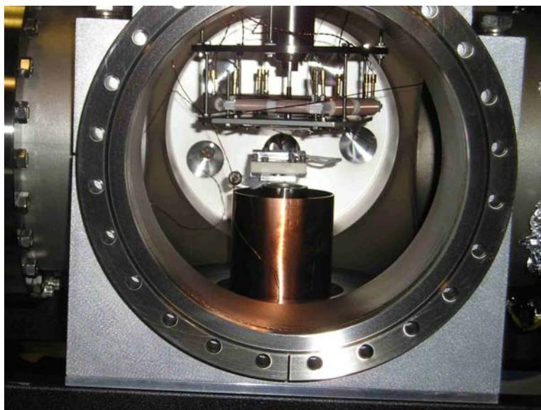
Fig. 1. View of the electron gun, beam tube, detector, manipulator arm, cryostat and thermal shield.
