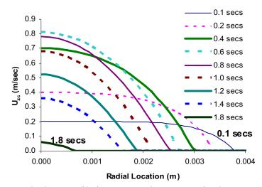
Axial velocity profile for constant inlet pressure of 20 kPa (Mold temperature =  $400^{\circ}$ C, initial melt temperature =  $1500^{\circ}$ C, interfacial heat transfer coefficient =  $2,000 \text{ W/m}^2$ -K).
