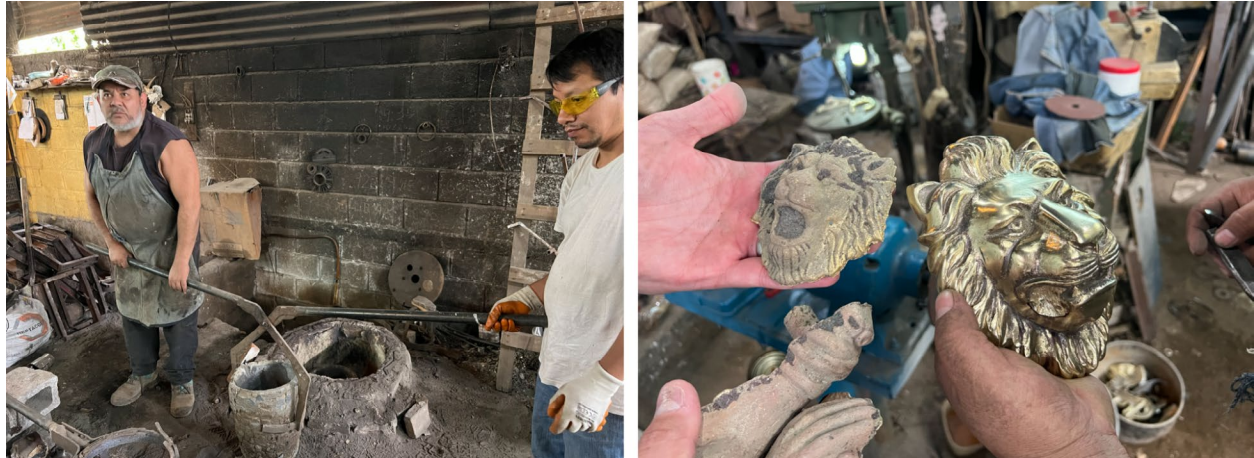
Figure 4, Left. Dany Tinoco and Carlos Cabrera lift a crucible from the furnace to begin the casting process. (Figure 5, Right) Rough bronze casting versus finished and polished casting. Photo by Juan Noguera.
