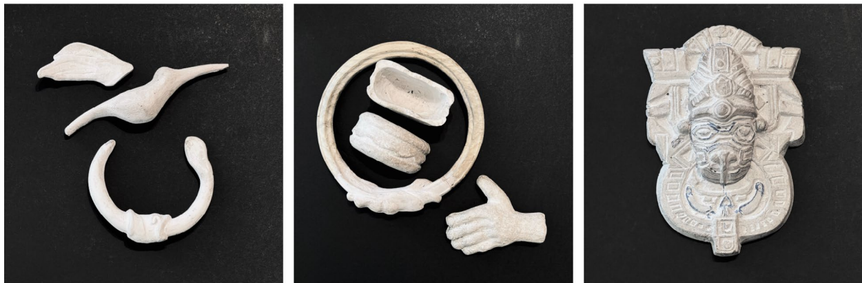
Figure 3. Forms created by artisans in preparation for sand casting of bronze. These objects are a combination of wooden forms, plaster, clay, and automotive body filler. Photographs by Juan Noguera.
