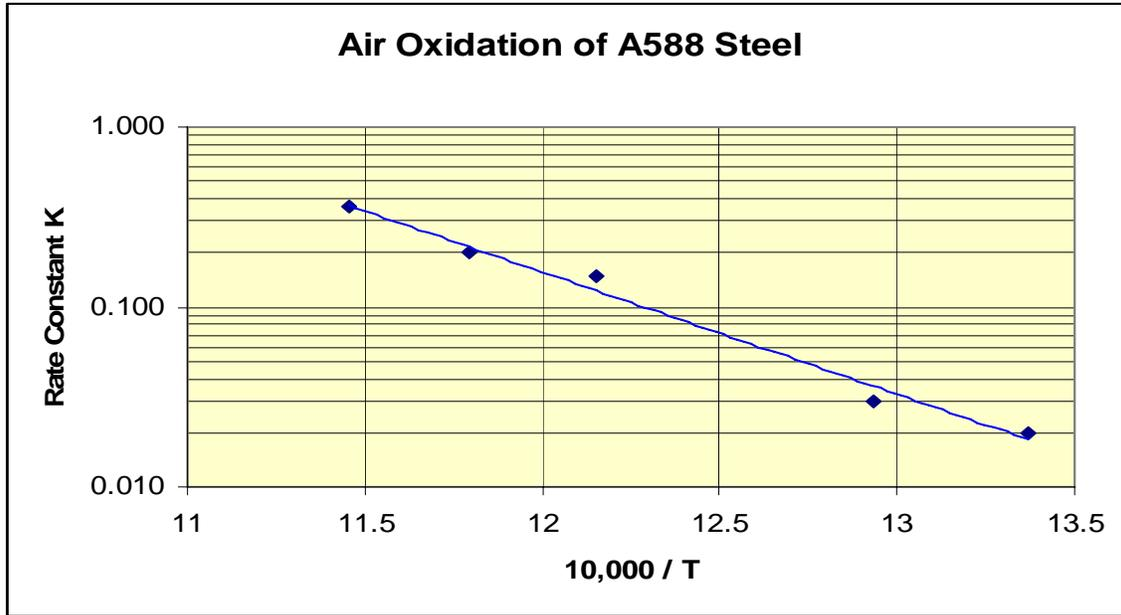
Figure 2. Plot of measured rate constants in ( $\text{mg}/\text{cm}^2 \text{ hour}^{1/2}$ ) vs. inverse of the absolute temperatures, for dry air oxidation of the A588 steel, at 475, 500, 550, 575 and 600 °C.
