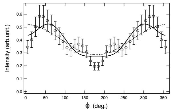
FIG. 3. Comparison between the angular distribution measured for parallel transitions (data points with statistical error bars) and fits obtained using Eq. (5) with  $P = 1.0$  (dashed curve) and Eq. (7) with  $P = 0.85$  (solid curve).
