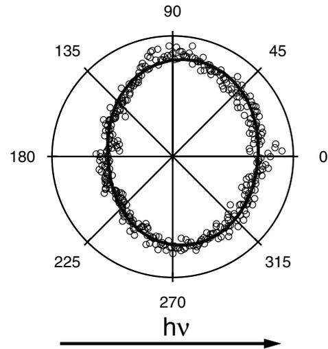
FIG. 1. Azimuthal dependence of the angular distribution for  $N$   $1s$  photoelectrons emitted from randomly oriented molecules at 660 eV photon energy (open circles) and fit obtained with Eq. (4) (solid curve). The photon propagation direction corresponds to the  $180^\circ \rightarrow 0^\circ$  axis.
