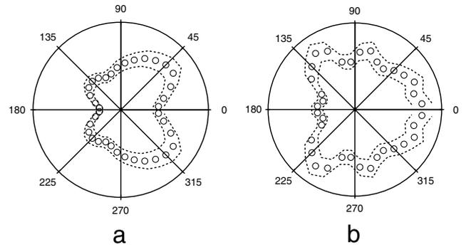
FIG. 2. Photoelectron angular distributions measured for parallel (a) and perpendicular (b) molecular orientations at 660 eV photon energy. The dashed lines represent the statistical error. In (a) the molecular axis points out of the paper, while in (b) the molecular axis is aligned along the 90°–270° axis.
