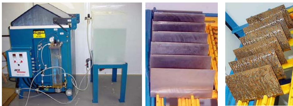
Figure 13 (top left). Exposure chamber and solution reservoir used for salt spray tests.
