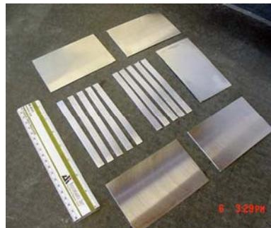
Figure 12. Coupon specimens for laboratory immersion and salt spray tests for rock bolts and I-beams. Similar specimens have to be prepared for the new specimens proposed in this study.
