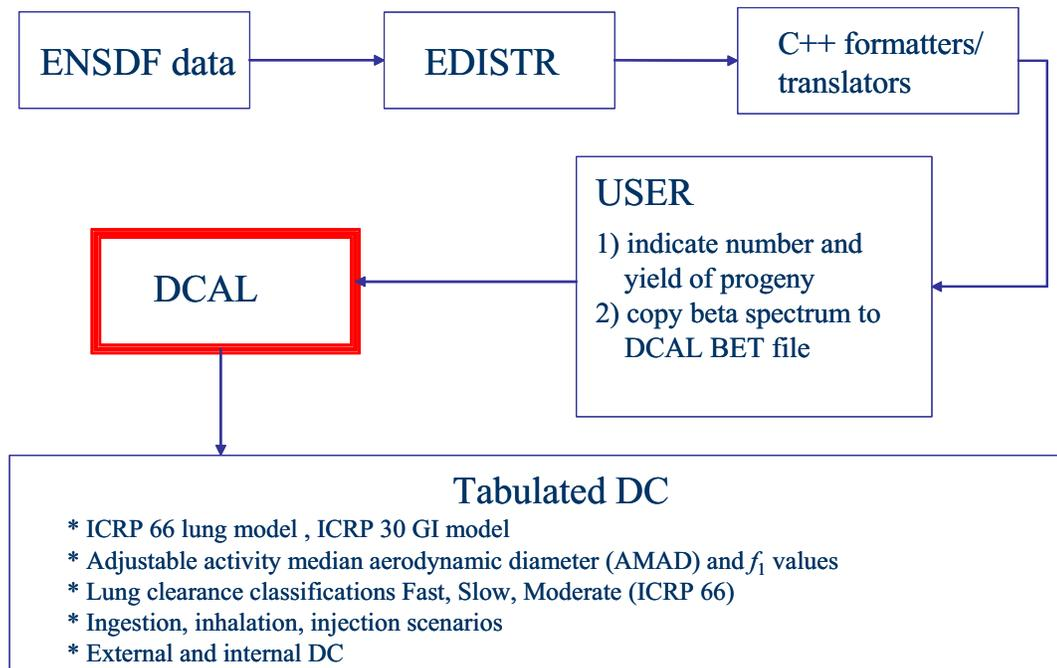
*Dose Coefficient Working Group Methodology Flow Sheet. The ENSDF code is used to obtain nuclear physics data. The EDISTR code prepares the data for input into the dose calculation code DCAL.*
