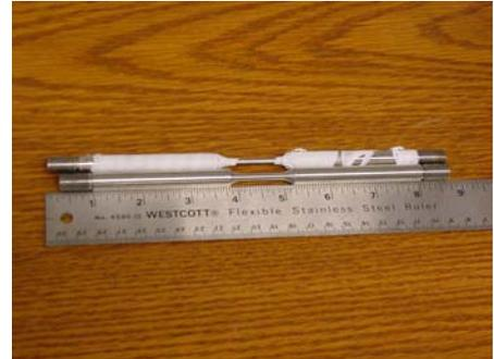
Figure 9. Stress strain plot of the alloy 22 in wrought condition. A photo of the specimens before and after the pulling in YM 100x water electrochemical environment are shown (right side). Please note the difference in the length the specimen before and after loading.
