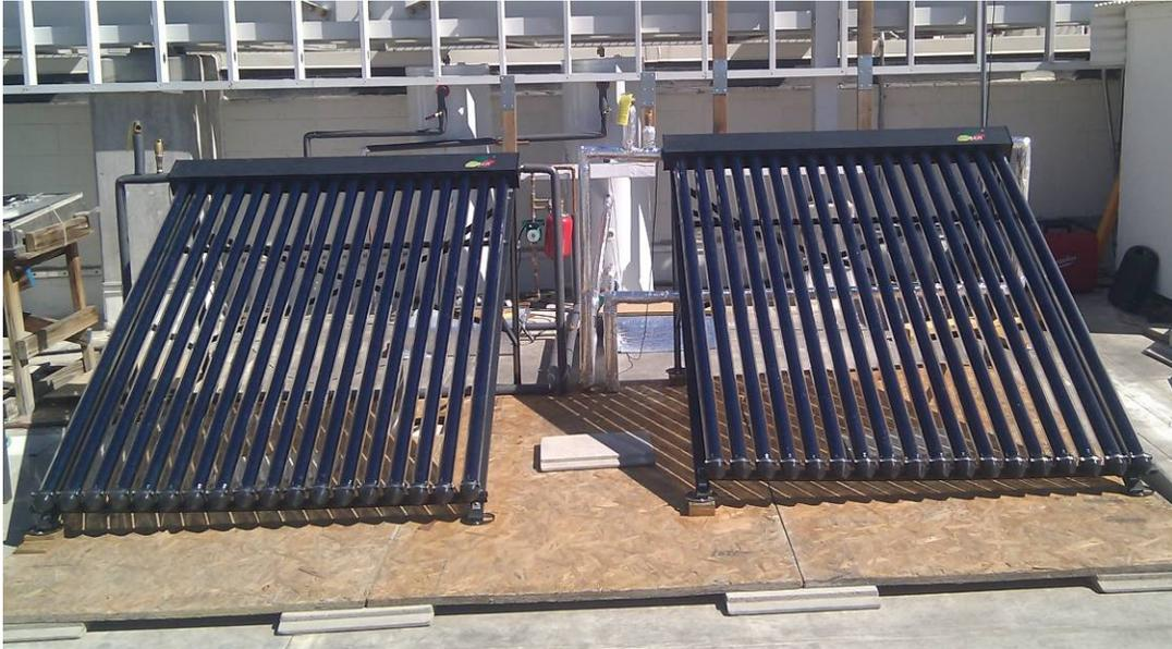
**Figure 2. Solar water heaters being tested**
