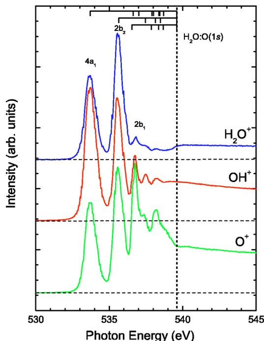
FIG. 2. Comparison of the positive-ion yields for three positive ions: the parent ion  $\text{H}_2\text{O}^+$  and two of the stronger fragments  $\text{OH}^+$  and  $\text{O}^+$ . For visualization purposes, the intensity scale and the scaling between the shown fragment ions is purely arbitrary.
