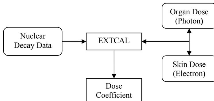
Figure 2.3.4.2. Schematic of DCAL's dosimetric system for the computation of an external dose coefficient calculation.
