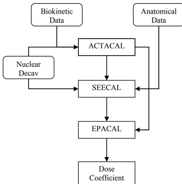
Figure 2.3.4.1. Schematic of DCAL system for internal radiation dosimetry calculations—adopted from ORNL/TM-2001/190 (Eckerman et al. 2001)
