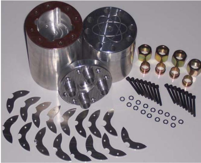
*Figure 1. Components of the CETON (Cooled Electron Target--Optimized for Neutron production) excluding tungsten-copper disks for converting electrons to photons. The W-Cu disks fit in the cavity at the upper left. In addition, the body is bored to accept a 10" aluminum-clad uranium photo-neutron generator.*
