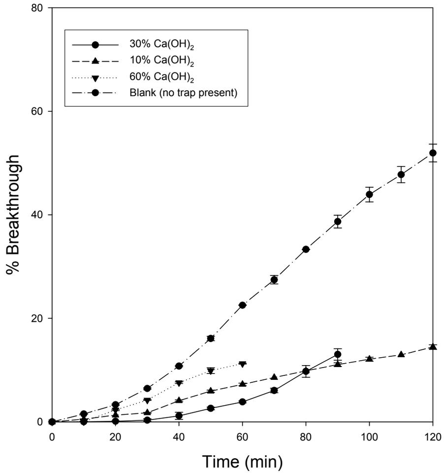
Figure 2: The breakthrough of iodine on 0.02 g of Ca(OH)<sub>2</sub>:sphagnum mixtures using the fuel rod simulator experiment described in earlier reports. The flow rates were 20.0 ml/min.
