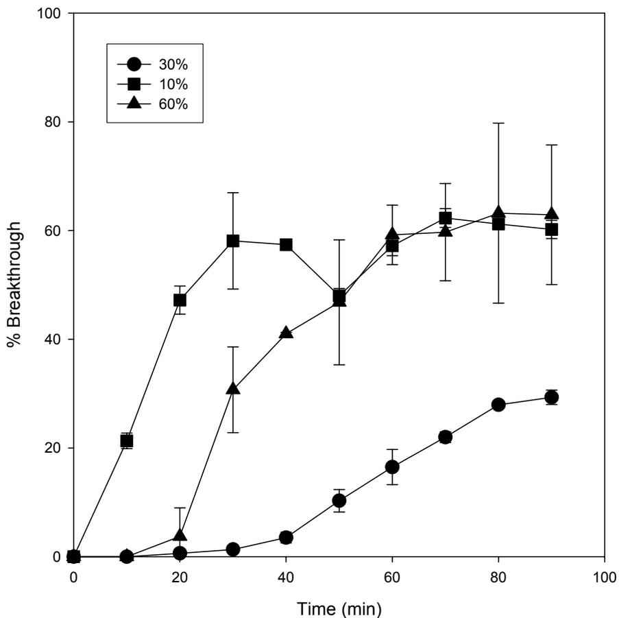
Figure 1: The breakthrough of iodine using the iodine generator apparatus described in earlier reports. The trap consisted of 0.5 g of  $\text{Ca}(\text{OH})_2$ : sphagnum mixtures. Three ratios were tested: 10, 30, 60%. The flow rates were 20.0 mL/min and the concentration of iodine was  $\sim 10^{-5}$  mol/L. The carrier was 50% saturated with nitric acid vapor.
