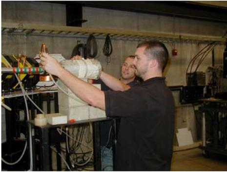
*UNLV graduate students Timothy Beller and Ryan LeCounte couple the UNLV High-Power RACE Target to a linear electron accelerator at the Idaho Accelerator Center.*
