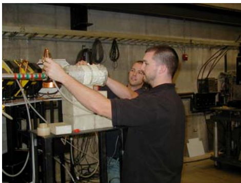
UNLV graduate students Timothy Beller and Ryan LeCounte couple the UNLV High-Power RACE Target to a linear electron accelerator at the Idaho Accelerator Center.
