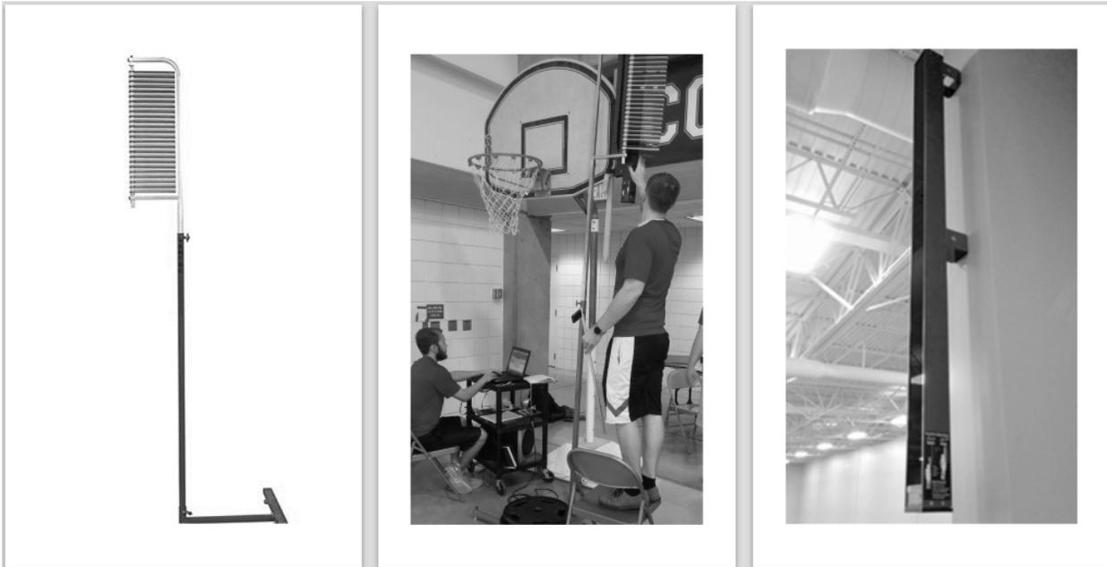
**Figure 1.** left picture is an example of a Vertec Vertical jump device, middle picture is an example of how the data collection was set, right is an example of a Brower Vertical Jump device.
