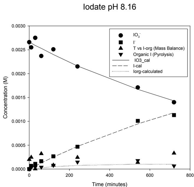
**Figure 12: Reaction of  $\text{IO}_3^-$  with sphagnum peat at 60°C at pH 8.16. I-org corresponds to the organic bound iodine (substitution) and was calculated by mass balance. Iodate and iodide were measured by ion chromatography.**
