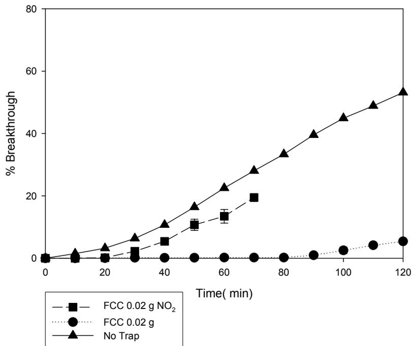
**Figure 24: The impact of NO<sub>2</sub> on iodine breakthrough on FCC using the fuel rod dissolution apparatus.**
