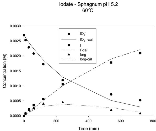
**Figure 11: Reaction of  $\text{IO}_3^-$  with sphagnum peat at 60°C at pH 5.2. I-org corresponds to the organic bound iodine (substitution) and was calculated by mass balance. Iodate and iodide were measured by ion chromatography.**
