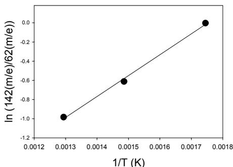
**Figure 19: Changes in the production of methyl iodide with temperature are a result in the higher activation energy for formation of dimethyl sulfide. This is analogous to the quaternary ammonium type resin discussed above.**
