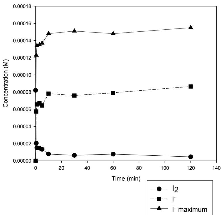
Figure 2: Reaction of iodine with vanillin (40 $\mu\text{M}$ ) at 25 $^\circ\text{C}$  and pH 2.5.
