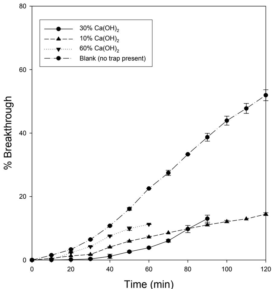
Figure 22: Effect of  $\text{Ca}(\text{OH})_2$  content on the efficiency of sphagnum during fuel rod dissolution simulations. All traps contained 0.02g of the sphagnum –  $\text{Ca}(\text{OH})_2$  combination.
