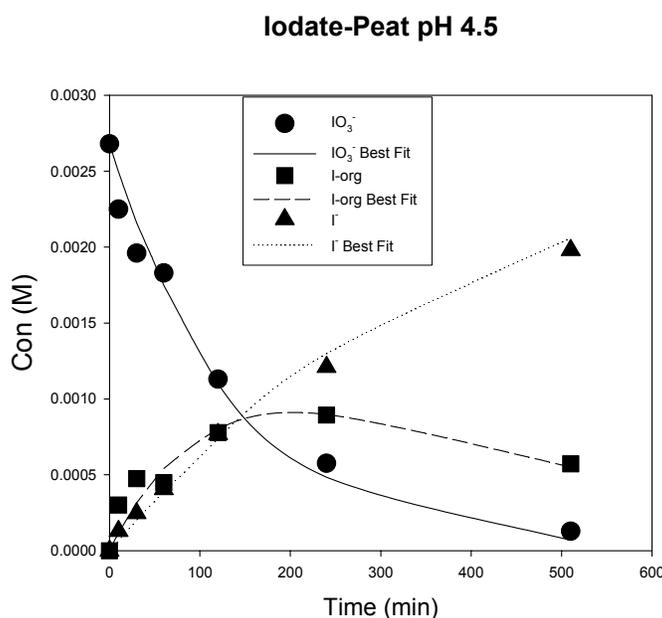
**Figure 10: Reaction of  $\text{IO}_3^-$  with sphagnum peat at 60°C at pH 4.5. I-org corresponds to the organic bound iodine (substitution) and was calculated by mass balance. Iodate and iodide were measured by ion chromatography.**
