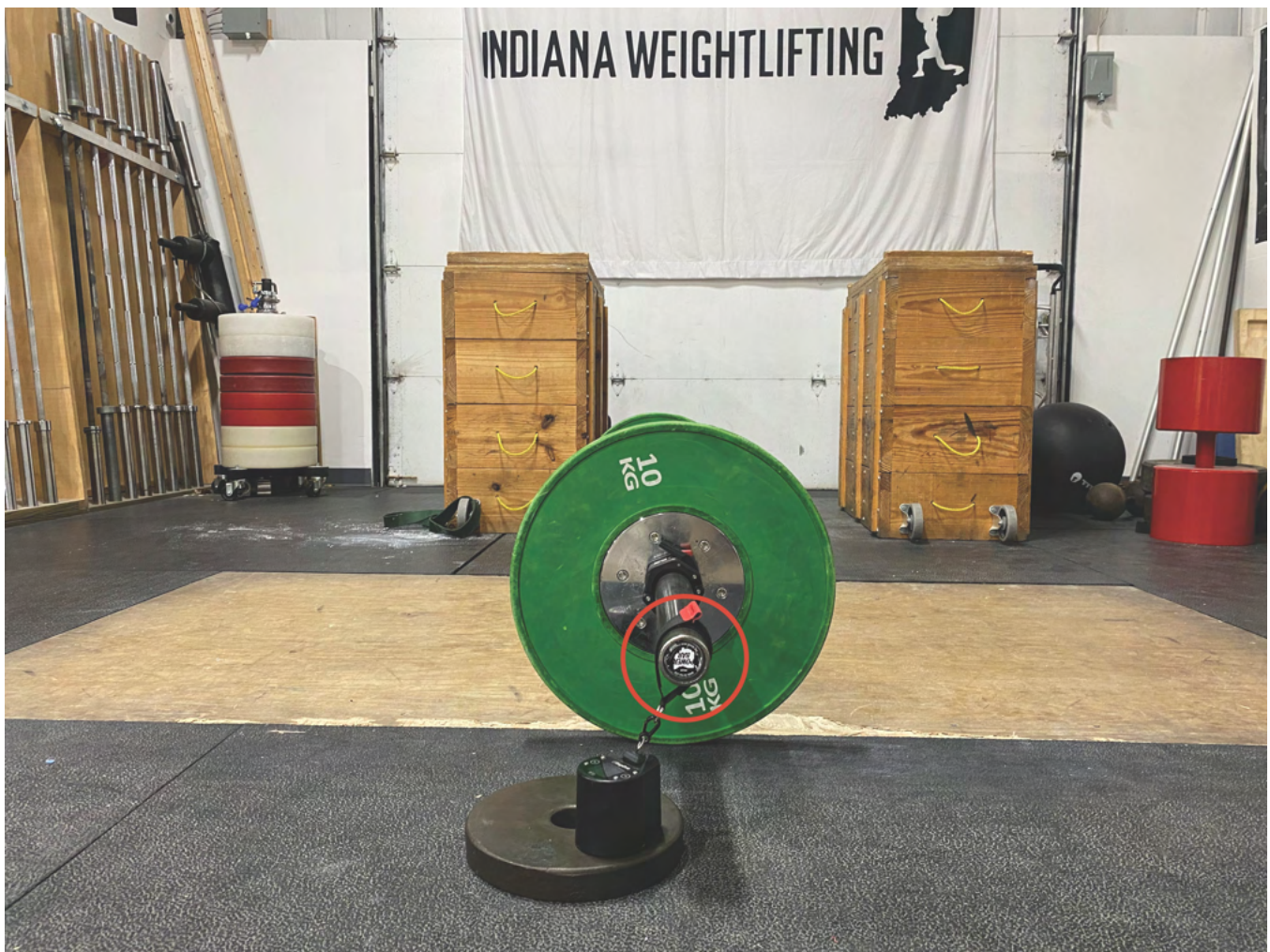
Figure 1. Linear Position Transducer (LPT) unit hooked to bar. Circle indicates tether attachment to bar.
