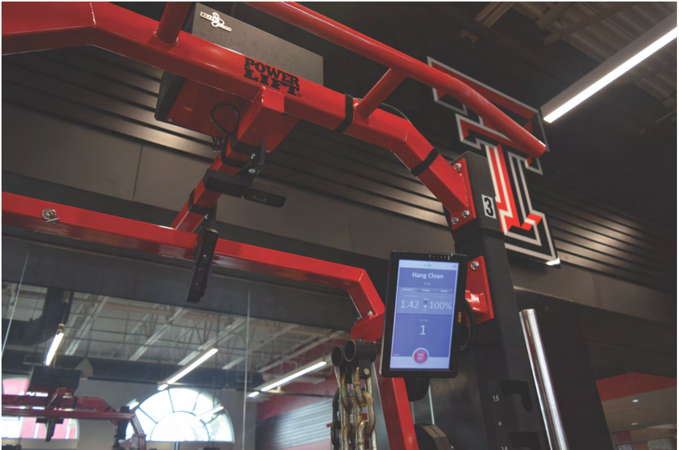
Figure 3. Camera-based system affixed to a power rack. Note the main unit above the rack, dual camera arrays mounted to the upper crossbeam, and touch panel video display mounted to the right upright.
