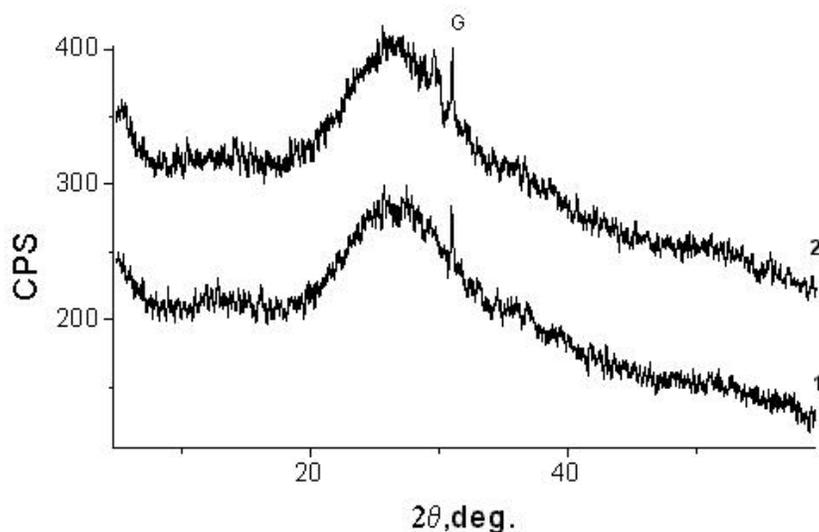
Figure 2. XRD patterns of iodine doped (432 mg/g) activated carbon after gamma-irradiation in nitrogen atmosphere at: 1)  $3.3 \times 10^7$  Rad and 2)  $2.1 \times 10^7$  Rad. Reflection of graphite phase is marked as (G).
