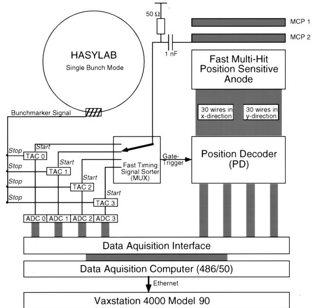
FIG. 1. Angle-resolved time-of-flight ion spectrometer with a position-sensitive anode including the electronic setup for data registration.
