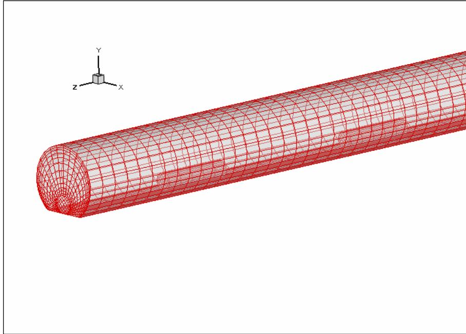
Figure 4-2. 3-D mesh for STAR-CD calculations (019RA.001)
