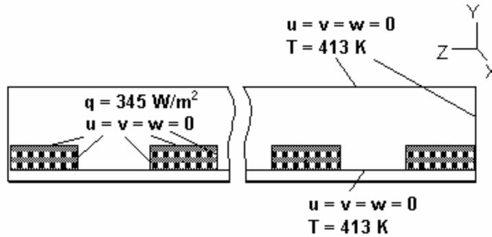
Figure 4-8. Boundary conditions for the natural convection calculations using STAR-CD for the post-closure period
