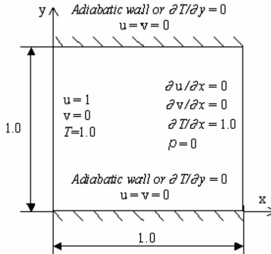
Figure 6-14 Computational domain with boundary conditions (UCCSN-SDR-001)
