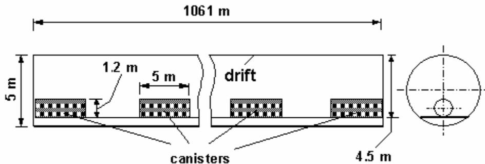
Figure 4-1. Dimensions of the drift and the canister
