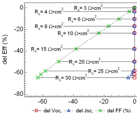
**Figure 8 Efficiency change with increasing  $R_s$ .**
