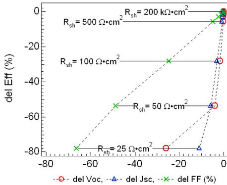
**Figure 7 Efficiency change with decreasing  $R_{sh}$ .**
