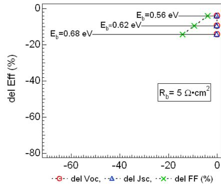
**Figure 6 Efficiency change with contact barrier increase.**
