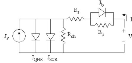
Figure 4 Two-diode solar cell discrete circuit model.
