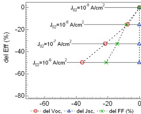
**Figure 9 Efficiency change with increasing  $J_{02}$ .**
