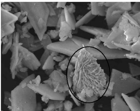
Figure 1: SEM image of hydroxyapatite synthesized containing strontium nitrate using the reflux method showing two different phases.
