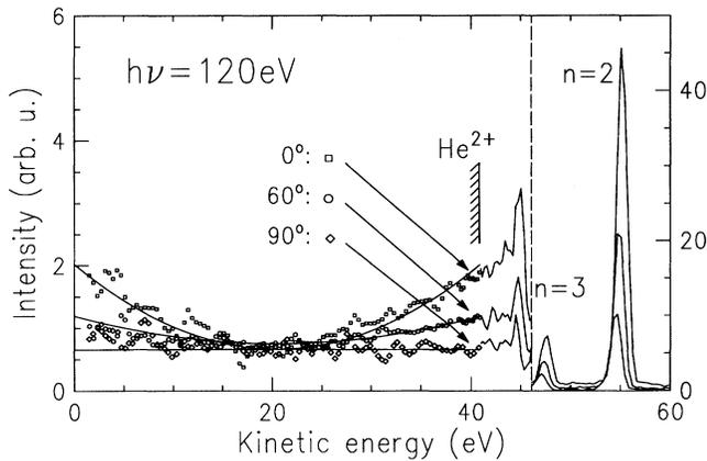
FIG. 4. Helium photoelectron spectra taken at  $h\nu=120$  eV at different angles with respect to the plane of the storage ring. The solid lines in the shake-off region are parabolic curves fitted to our spectra disregarding short-range variations which proved to be accidental.
