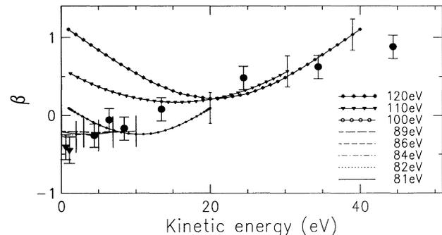
FIG. 6. Shake-off  $\beta$  curves at various photon energies as shown in Fig. 5(a) together with  $\beta$  values of the satellite  $n=4$  (solid circles) on its kinetic energy scale. The triangles represent data from Heimann *et al.* [27].
