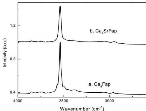
IR spectra of  $\text{Ca}_3\text{Fap}$  and  $\text{Ca}_4\text{SrFap}$  after annealing.
