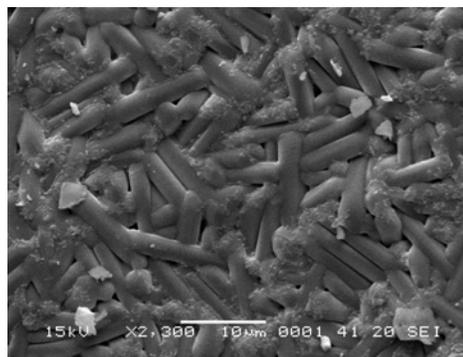
SEM micrograph of  $Ca_4SrFap$  (annealed sample)
