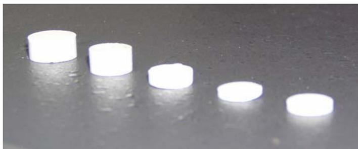
*MgO-ZrO<sub>2</sub> pellets synthesized from precipitation of metal salts.*
