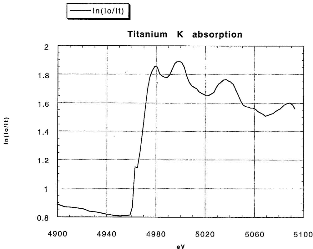
FIG. 3. Titanium *K* absorption spectrum measured without using an intensity feedback system.
