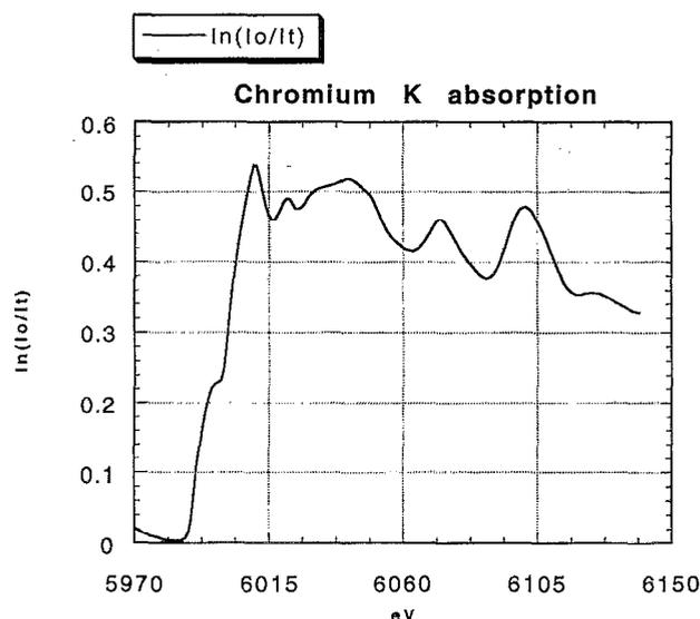
FIG. 2. Chromium *K* absorption spectrum measured without using an intensity feedback system.
