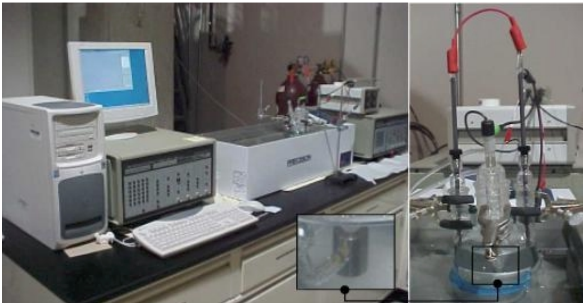
Figure 2. Electrochemical Polarization Test Setup
