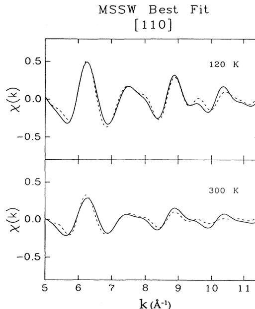
FIG. 7. The best fits of the MSSW calculations (dashed curves) to the filtered (10.0 Å) ARPEFS data (solid curves) for the [110] geometry at two temperatures, 120 and 300 K.
