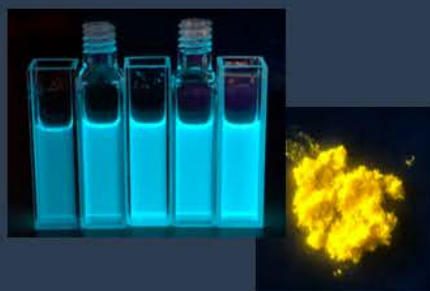
Figure 3. Serial dilutions in methanol ( 10^{-5} M) and solid state of p - \text{C}_9 -styryl pyridinium OTs showing fluorescence under UV-light.
