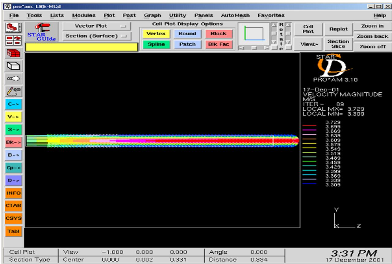
FIG-2: VELOCITY PROFILE ALONG AN AXIAL SECTION OF THE PIPE
