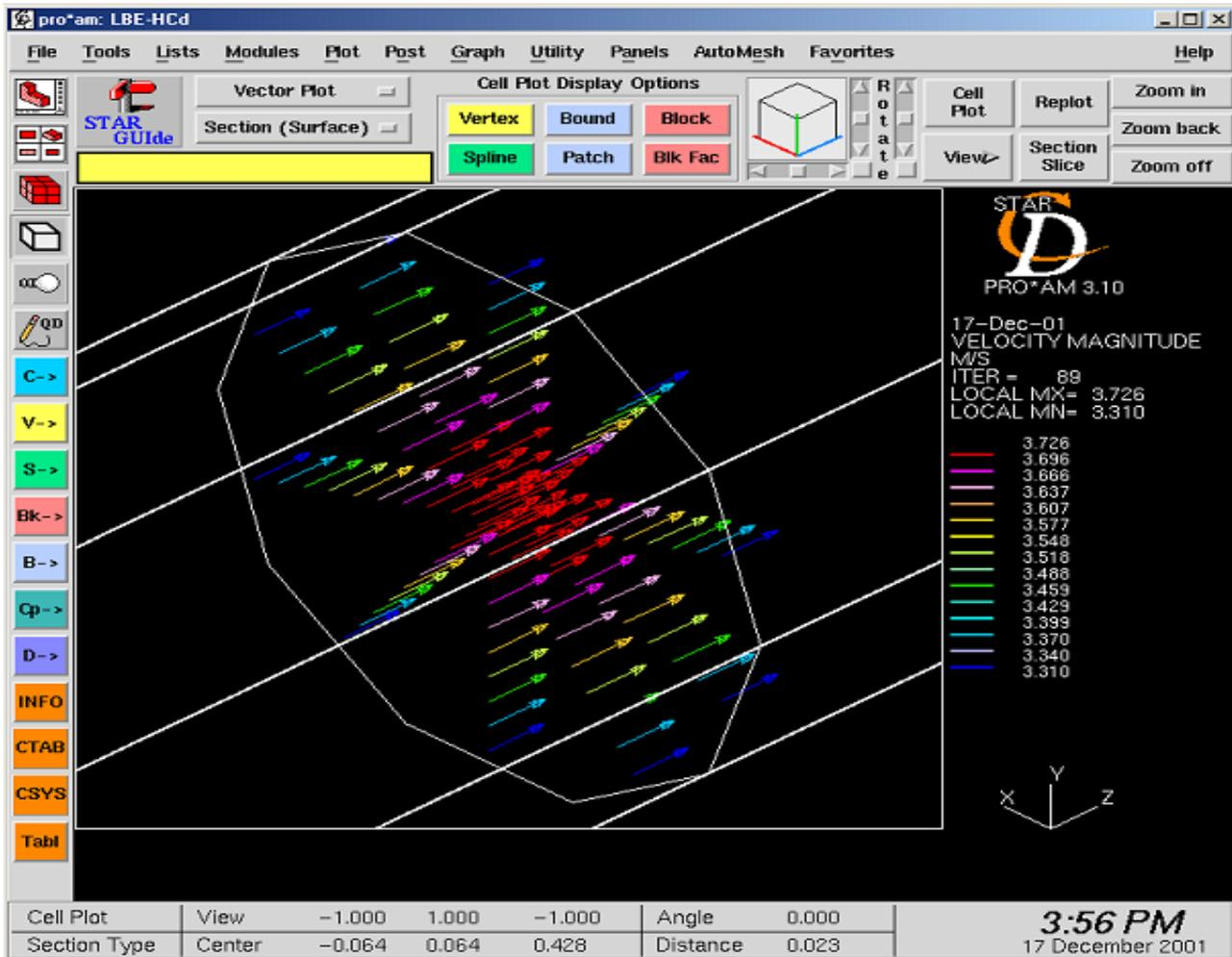
FIG-3: VELOCITY PROFILE ALONG THE DIAMETRICAL SECTION OF THE PIPE
