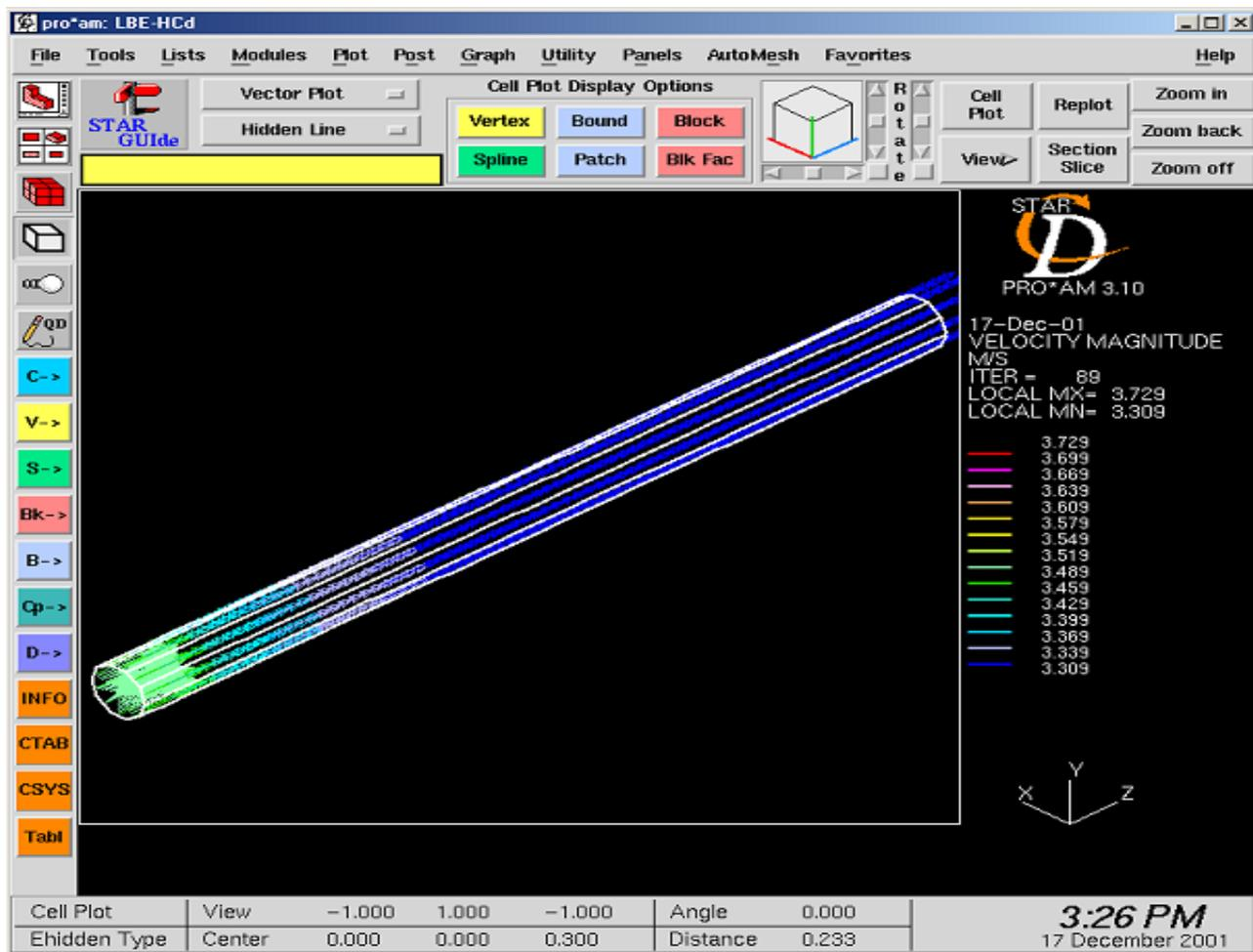
FIG-1: VECTORIAL REPRESENTATION OF THE VELOCITY OF THE FLUID IN THE PIPE
