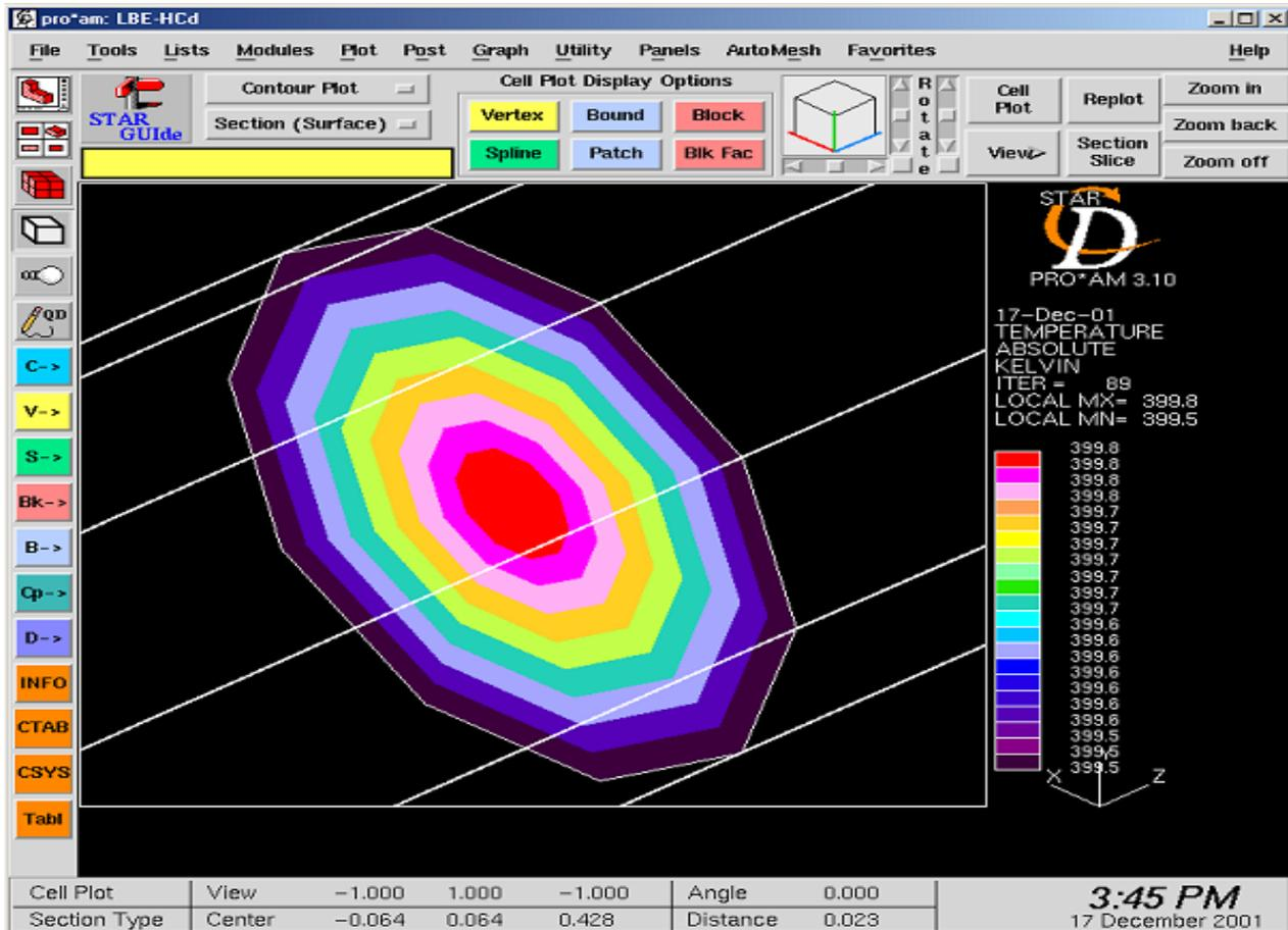
FIG-5: TEMPERATURE VARIATION ALONG A DIAMETRICAL SECTION OF THE PIPE
