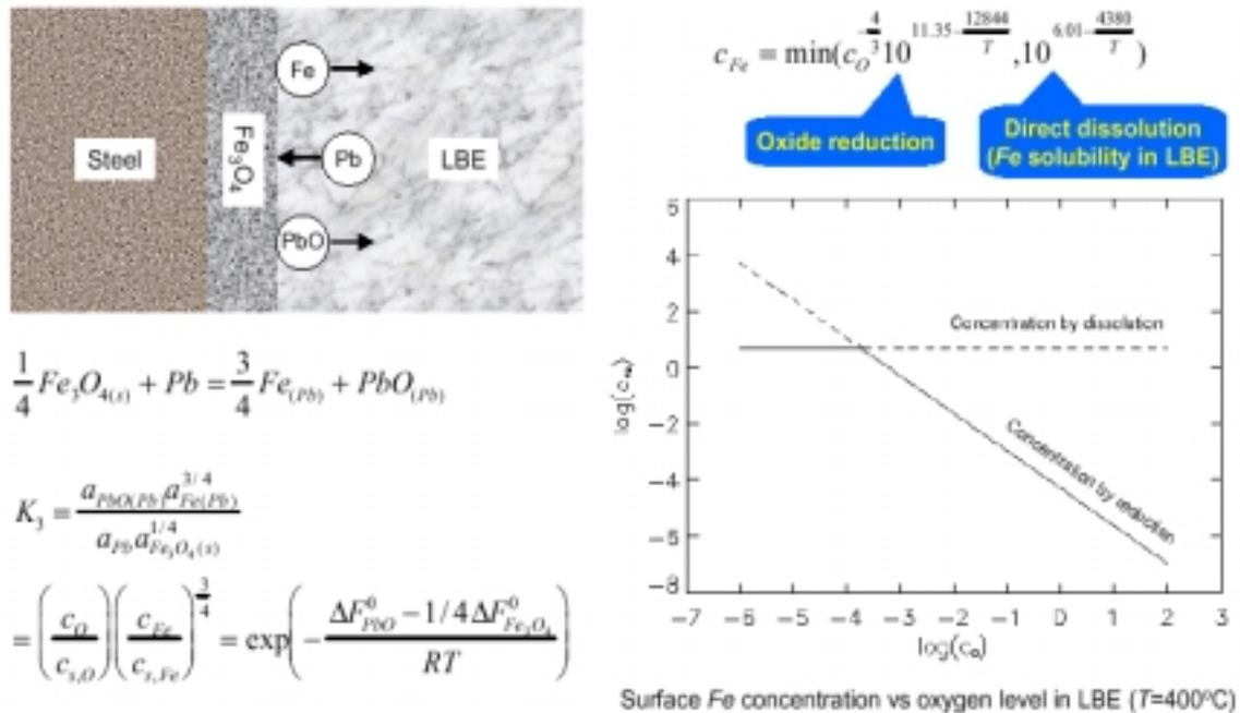
FIG-7: POSSIBLE REACTIONS BETWEEN IRON OXIDES AND LEAD AS PRESENTED IN A RECENT PAPER BY DR. NING LI et al. ANS CONFERENCE RENO 2001
