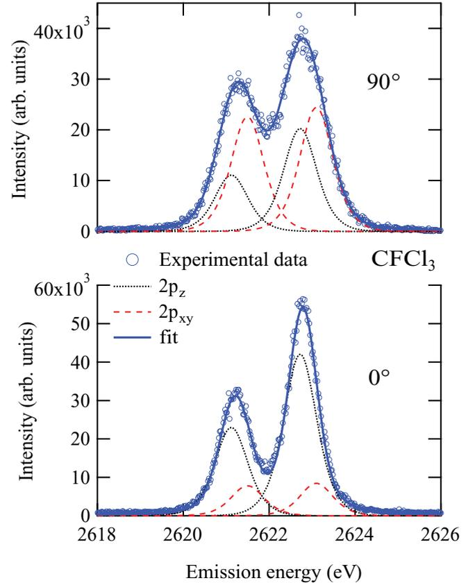
FIG. 7. (Color online)  $2p_z$  and  $2p_{x,y}$  subcomponents of the spin-orbit doublet in  $KL$  emission from  $\text{CFCl}_3$  as a function of polarization angle. Incident photon energy was set at the maximum of the  $\text{Cl}1s \rightarrow 12a_1$  resonance.
