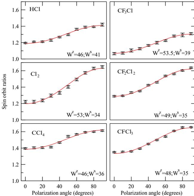
FIG. 8. (Color online) Spin-orbit ratios and electronic-state populations for various molecules measured as a function of polarization angle  $\chi$ . Circles are experimental data, and solid lines are fits using Eq. (10). Electronic-state populations are given in Table III.
