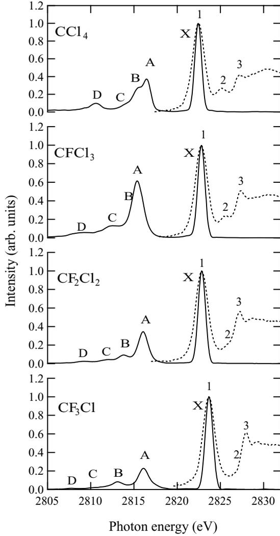
FIG. 4. Absorption (dashed) and  $KV$  emission spectra (solid) for  $\text{CCl}_4$ ,  $\text{CFCl}_3$ ,  $\text{CF}_2\text{Cl}_2$ , and  $\text{CF}_3\text{Cl}$ . Emission spectra are recorded at the maximum of the  $\text{Cl}1s \rightarrow \text{LUMO}$  resonances. Labels refer to assignments given in Table I.
