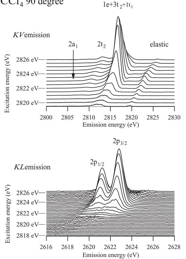
FIG. 3. *KV* and *KL* emission spectra from CCl<sub>4</sub> recorded at photon energies around the Cl1*s* → 7*a*<sub>1</sub> resonance ( $h\nu = 2822.5$  eV) at 90° with respect to the incident polarization.
