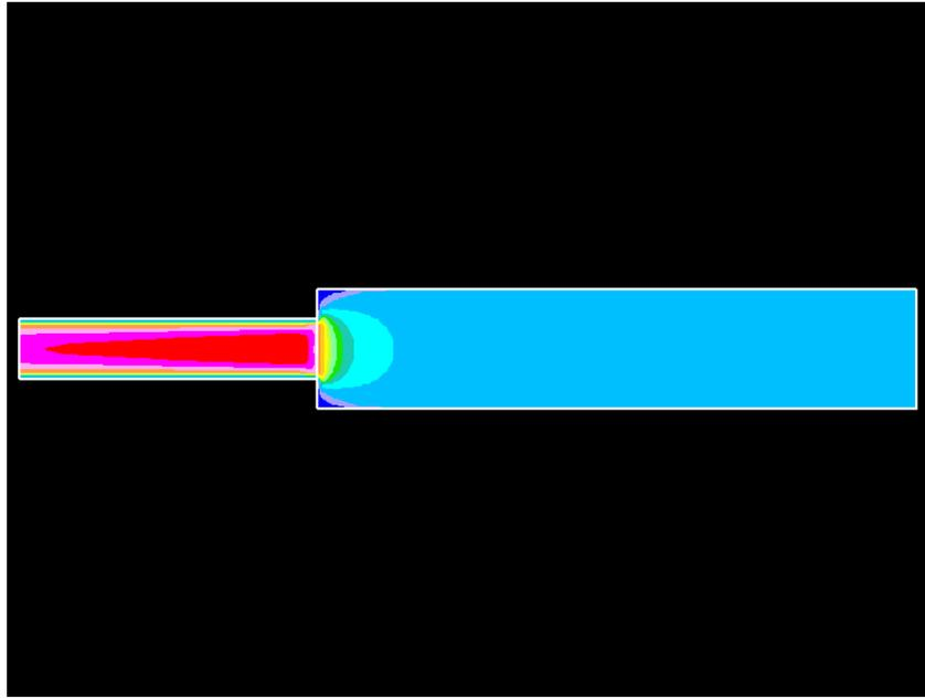
**Figure - 7:** Velocity magnitude for  $Re = 200,000$ (turbulent flow)
