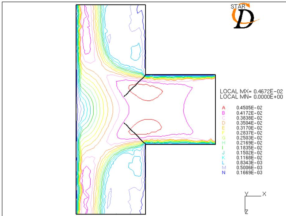
**Figure - 13:** Velocity lines for a middle inlet t-joint at  $Re = 2000$ (laminar flow)
