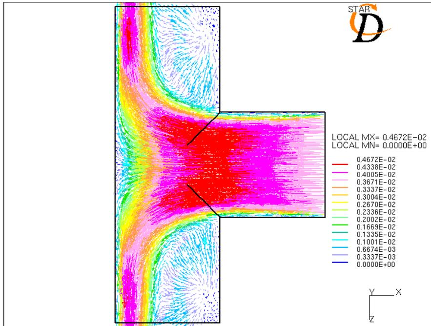
**Figure - 14:** Velocity vectors for a middle inlet t-joint at  $Re = 2000$ (laminar flow)
