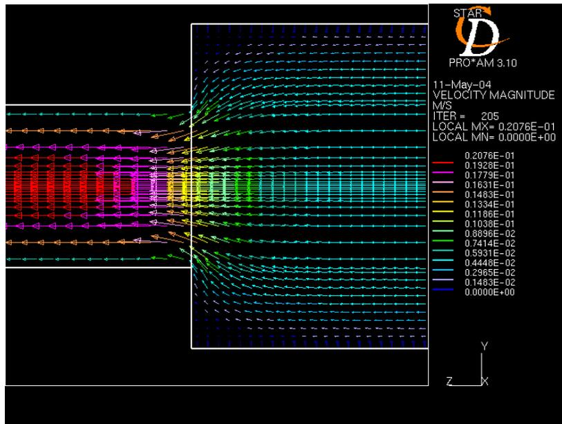
Figure - 6: Velocity vectors for  $Re = 2000$ (laminar flow)
