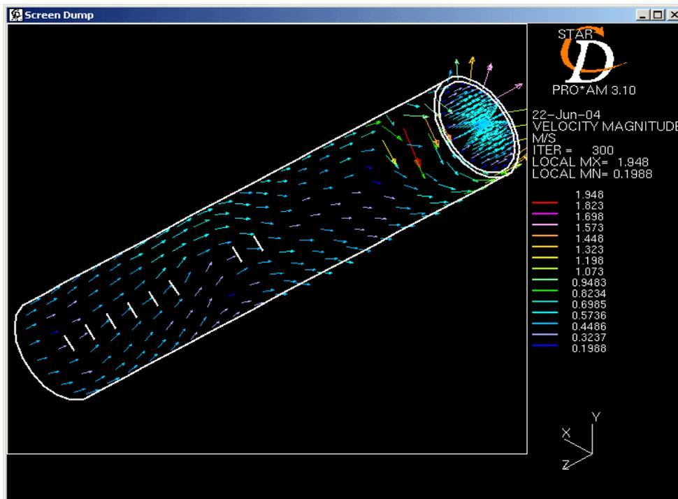
Figure 21 The velocity vector inside the pipe
