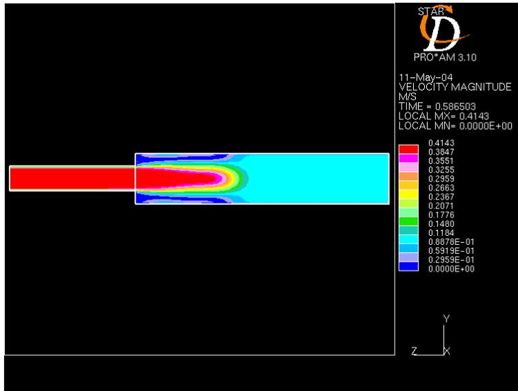
**Figure - 2:** Velocity plot for  $Re = 200,000$
