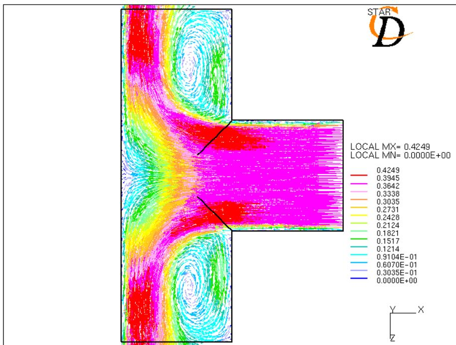
**Figure - 19:** Velocity vectors for a middle inlet t-joint at  $Re = 200,000$ (turbulent flow)
