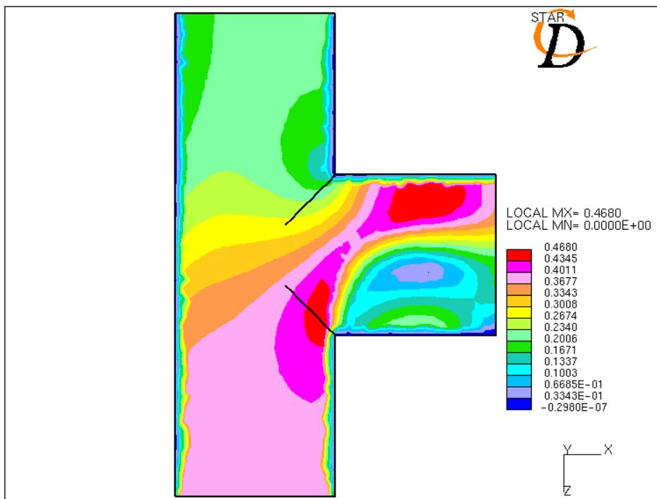
**Figure - 15:** Velocity magnitude for a side inlet(from bottom inlet) t-joint at  $Re = 200,000$ (turbulent flow)
