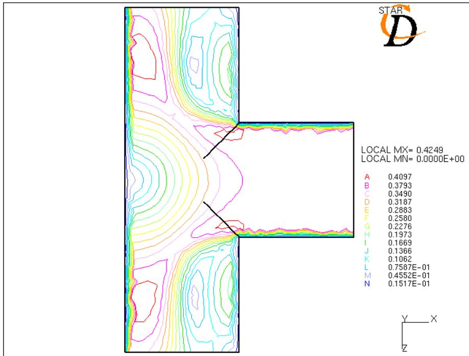
**Figure - 18:** Velocity lines for a middle inlet t-joint at  $Re = 200,000$ (turbulent flow)
