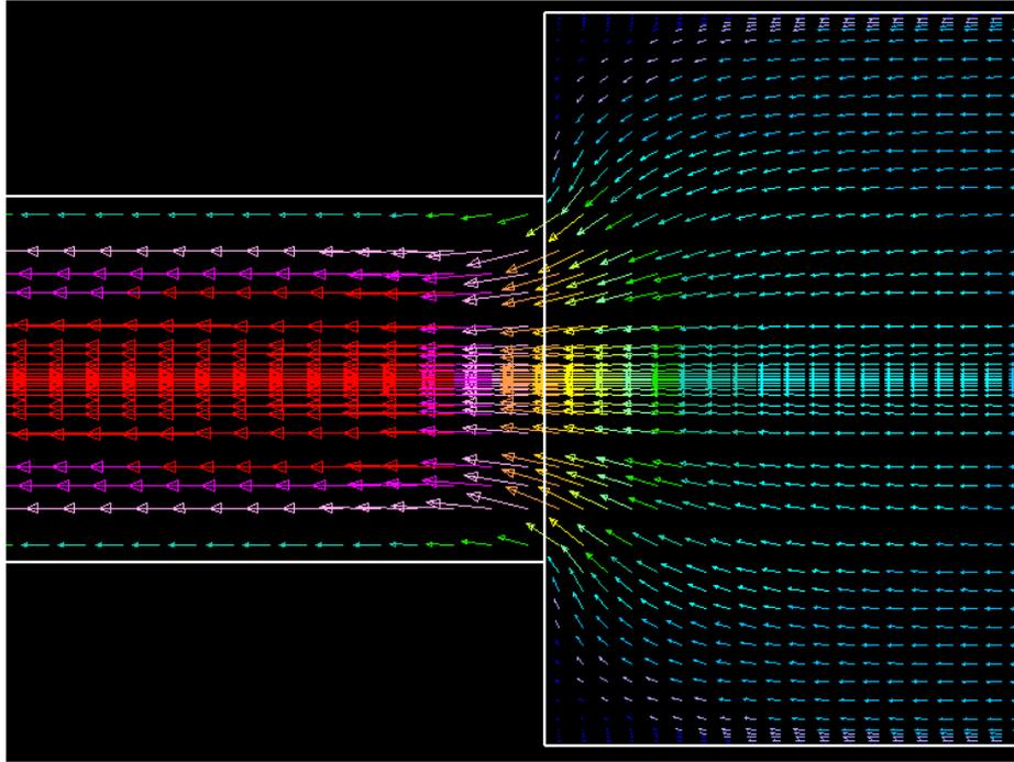
**Figure - 9:** Velocity Vectors for  $Re = 200,000$ (turbulent flow)
