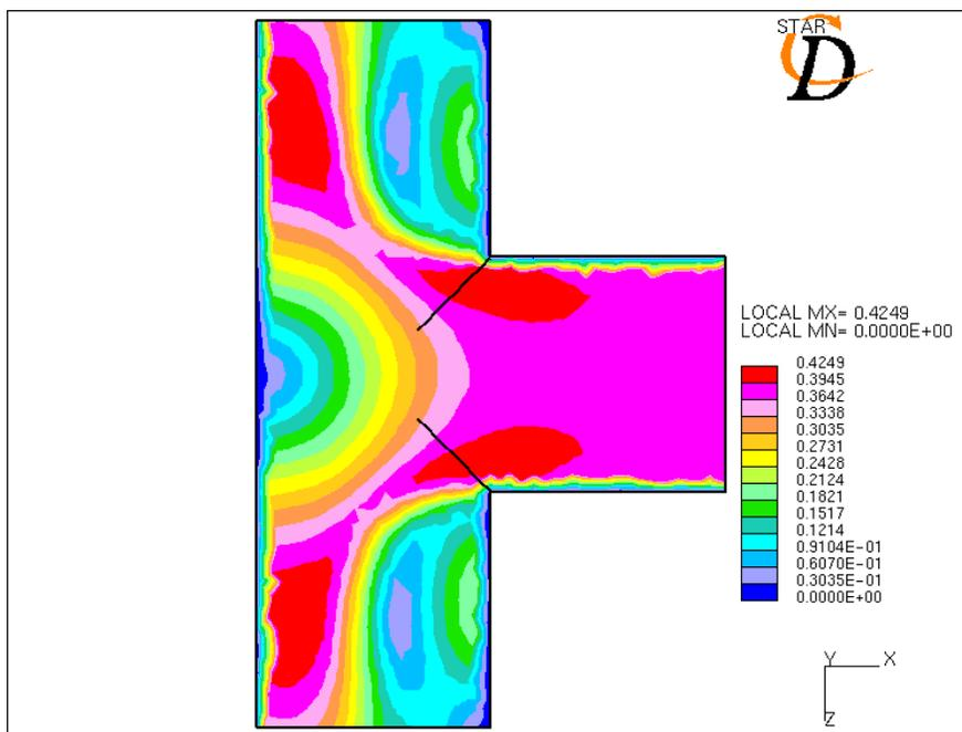
**Figure - 17:** Velocity magnitude for a middle inlet t-joint at  $Re = 200,000$ (turbulent flow)
