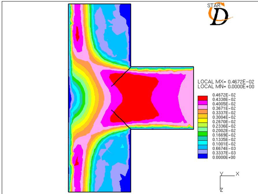
**Figure - 12:** Velocity magnitude for a middle inlet t-joint at  $Re = 2000$ (laminar flow)
