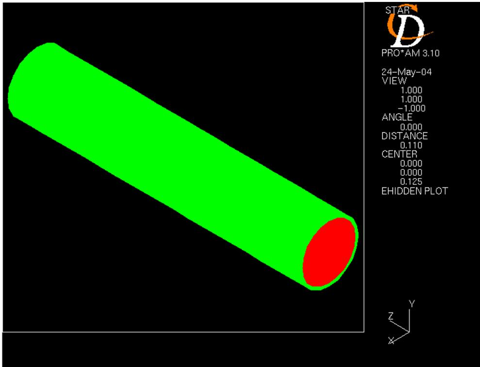
Figure 20 The 3-D CFD model (0.0508 m \* 0.25 m straight pipe )
