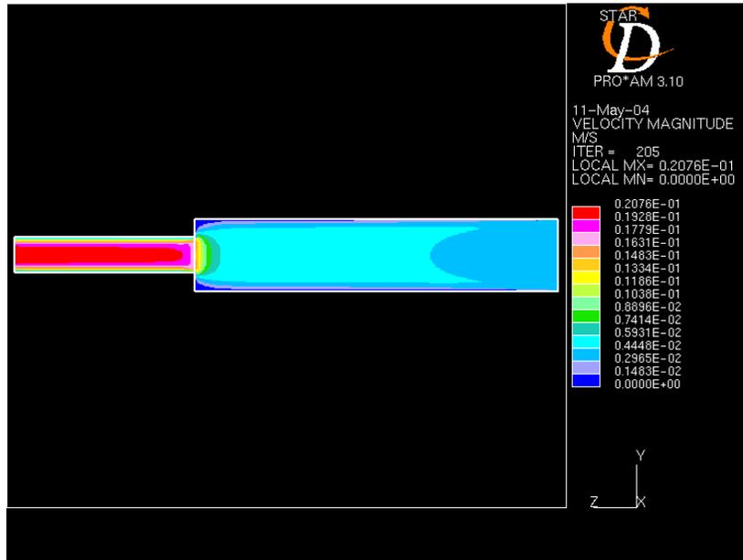
Figure - 5: Velocity plot for  $Re = 2000$ (laminar flow)
