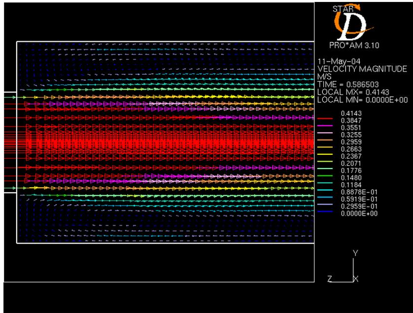
**Figure - 4:** Velocity vectors for  $Re = 200,000$
