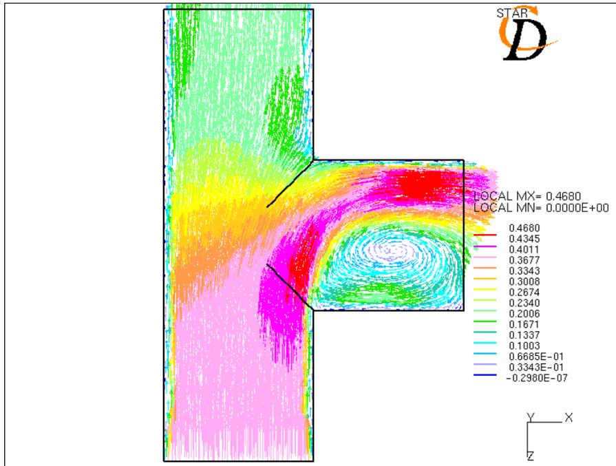
**Figure - 16:** Velocity vectors for a side inlet(from bottom inlet) t-joint at  $Re = 200,000$ (turbulent flow)
