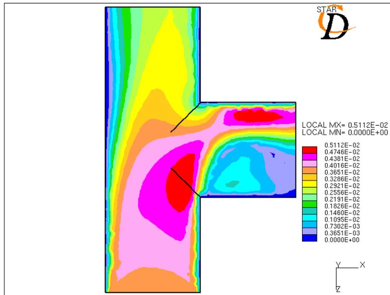
**Figure - 11:** Velocity magnitude for a side inlet(from bottom inlet) t-joint at  $Re = 2000$ (laminar flow)
