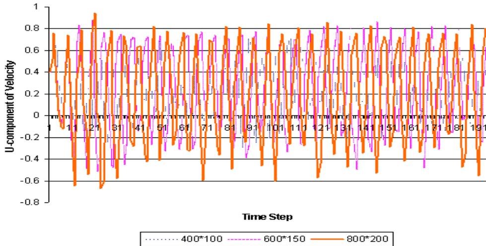
Figure – 41: U-component of velocity of point one in different sizes of mesh
