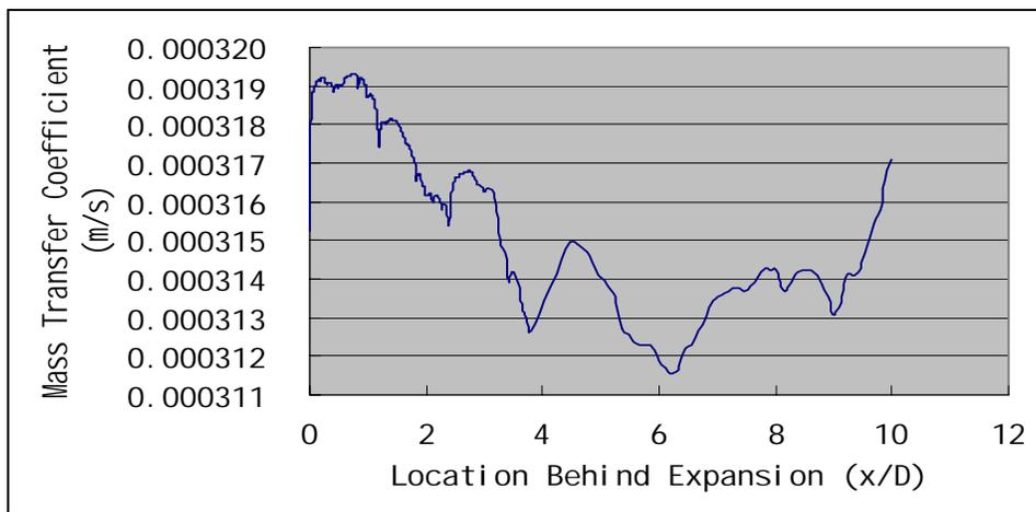
Figure – 44: Mass transfer coefficient variation at Re=24,000
