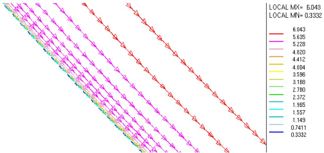
Figure 10: Velocity profile due to turbulent flow at the main test section in the closed toroidal loop model
