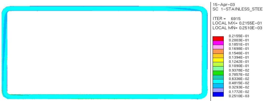
Figure 19: Concentration distribution for the laminar flow in the rectangular loop model
