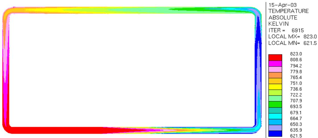
Figure 17: Temperature distribution for the laminar flow in the rectangular loop model
