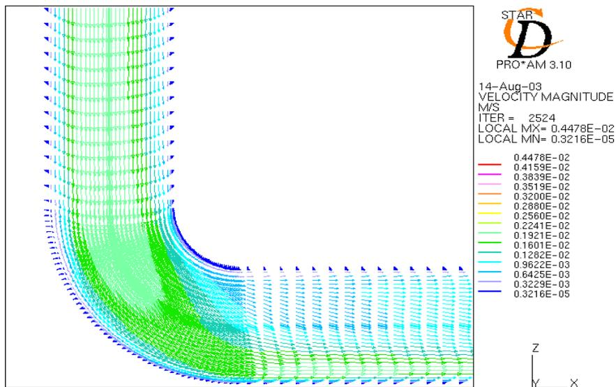
Figure 15: Velocity profile at an elbow section for the laminar flow in the rectangular loop model
