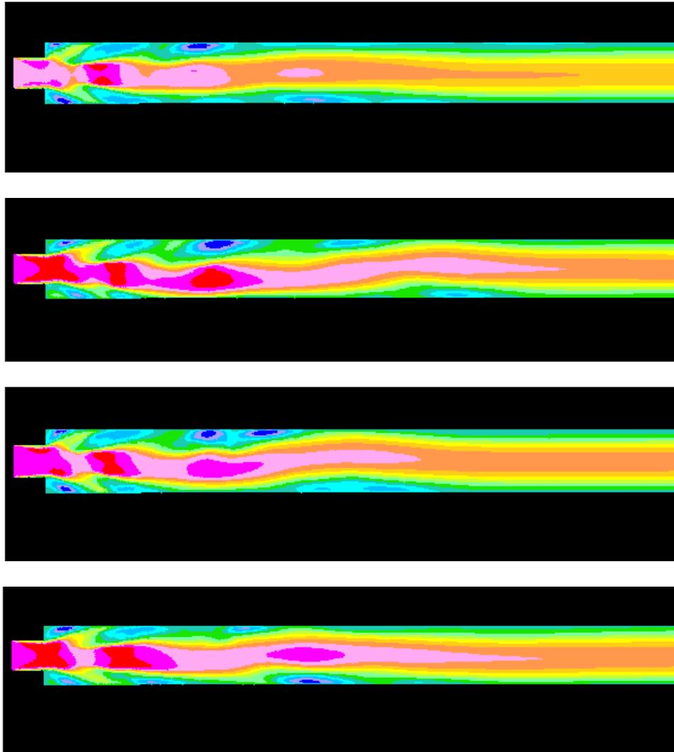
Figure – 40: Fluctuation of U-component of velocity
