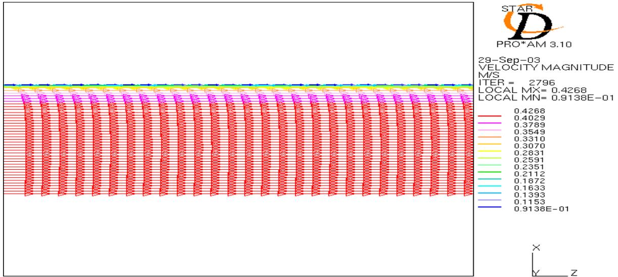
Figure – 4: Velocity Profile for the straight pipe model for a turbulent flow
