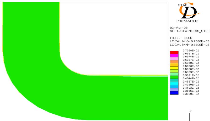
Figure 20: Concentration distribution for the laminar flow in the rectangular loop model
