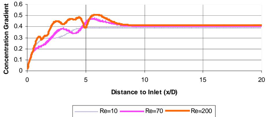
Figure – 34: Concentration gradient vs. distance to inlet at expansion ratio of 6
