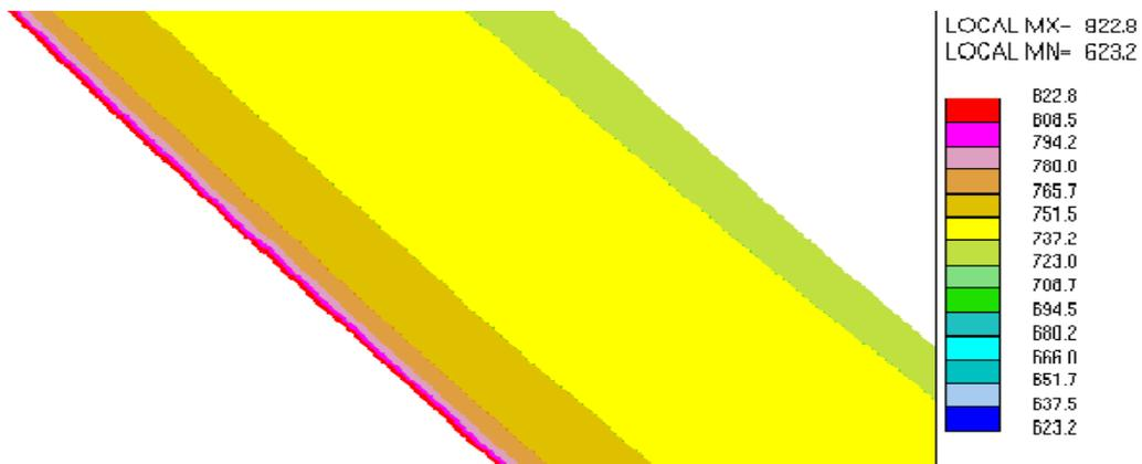
Figure 11: Temperature profile due to the turbulent flow at the main test section in the closed toroidal loop model
