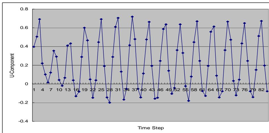
Figure – 39: U-component of velocity of monitored cell at Re equal to 1,000
