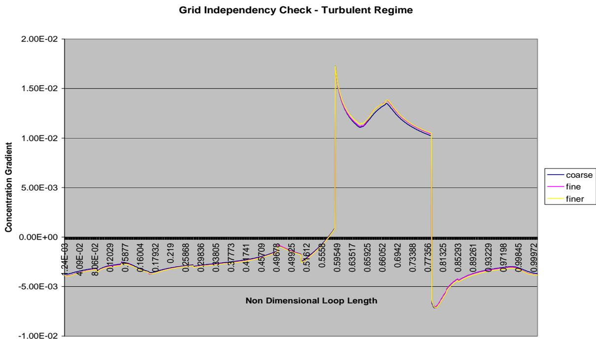
Figure – 23: Grid Independency Check for Turbulent Regime
