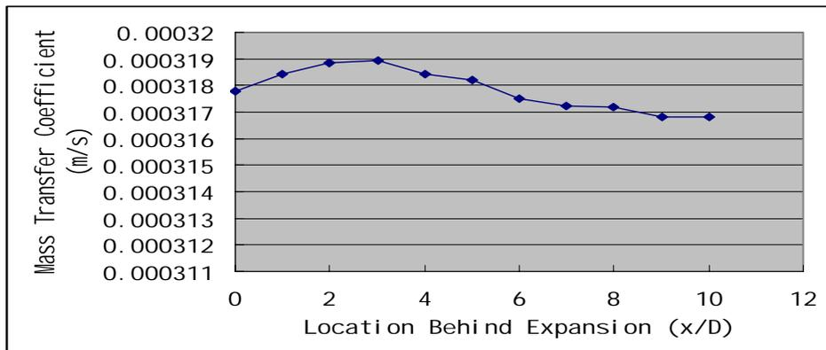
Figure – 46: Mass transfer coefficient variation at Re=24,000
