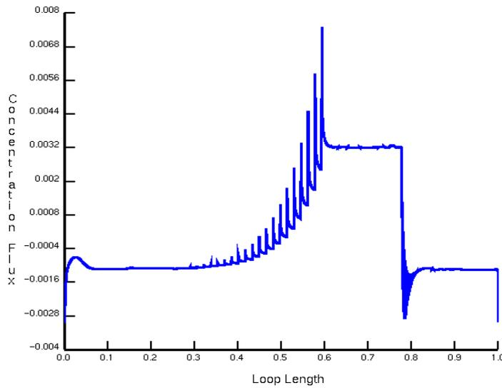
Figure 13: Corrosion/precipitation rate for the closed toroidal loop model
