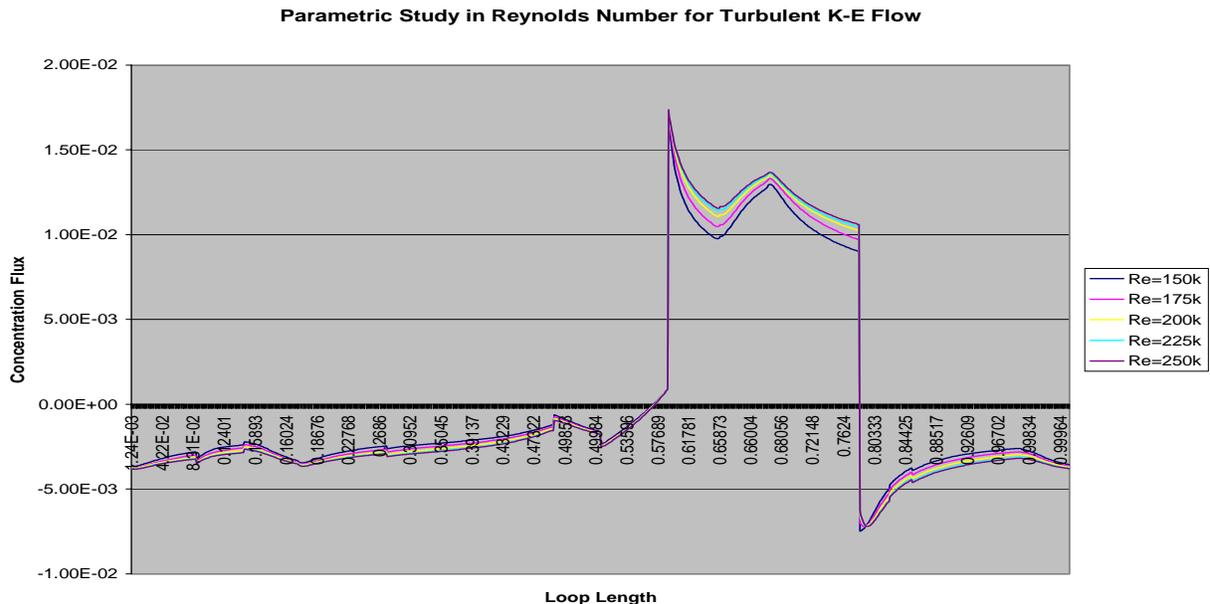
Figure – 24: Parametric Study in Reynolds Number for Turbulent K-ε Flow
