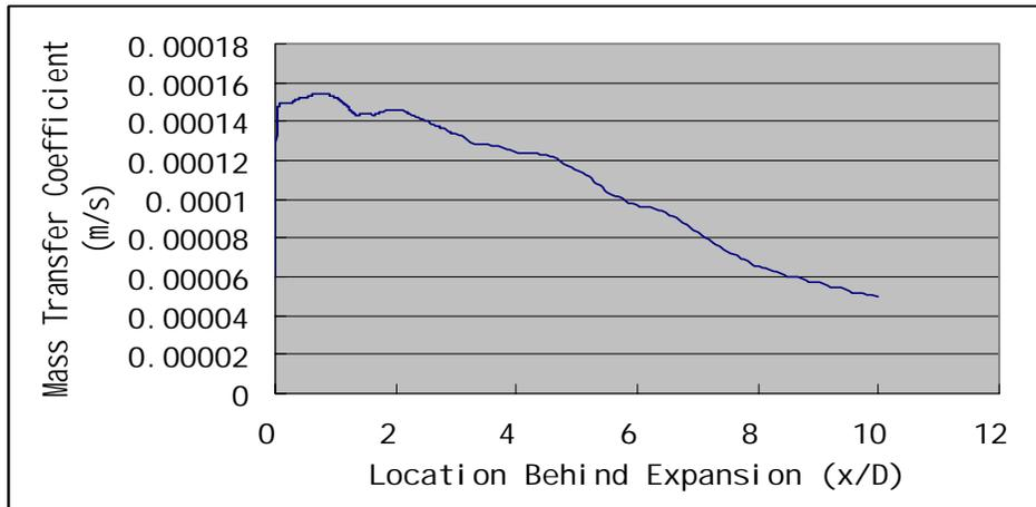
Figure – 43: Mass transfer coefficient variation at Re=1,000
