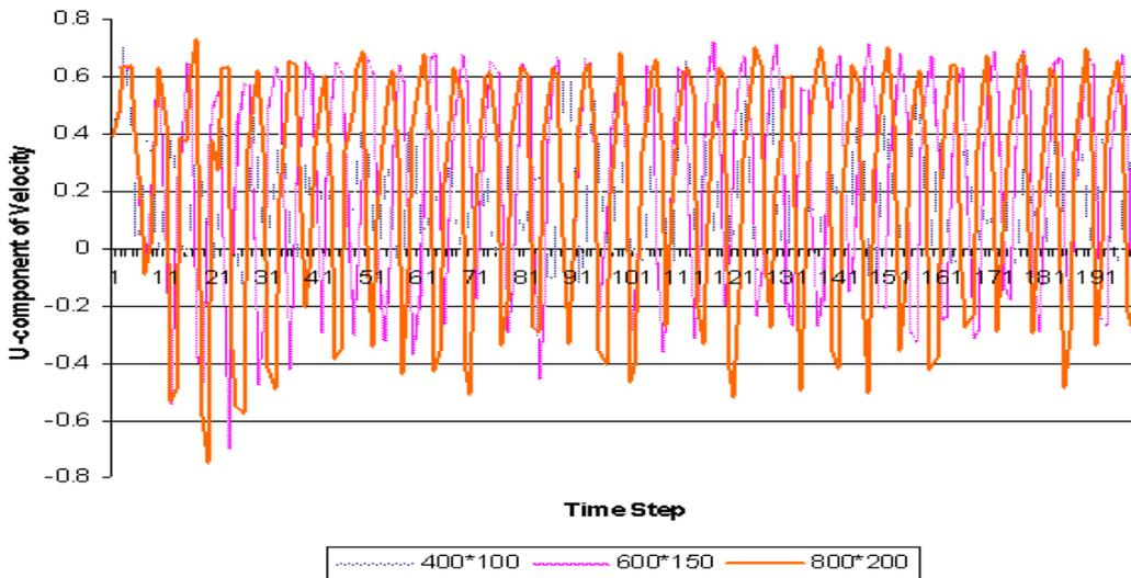
Fig – 42: U-component of velocity of point two in different sizes of mesh
