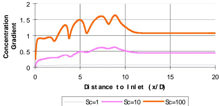
Figure – 37: Concentration gradient vs. distance to inlet at different Schmidt number
