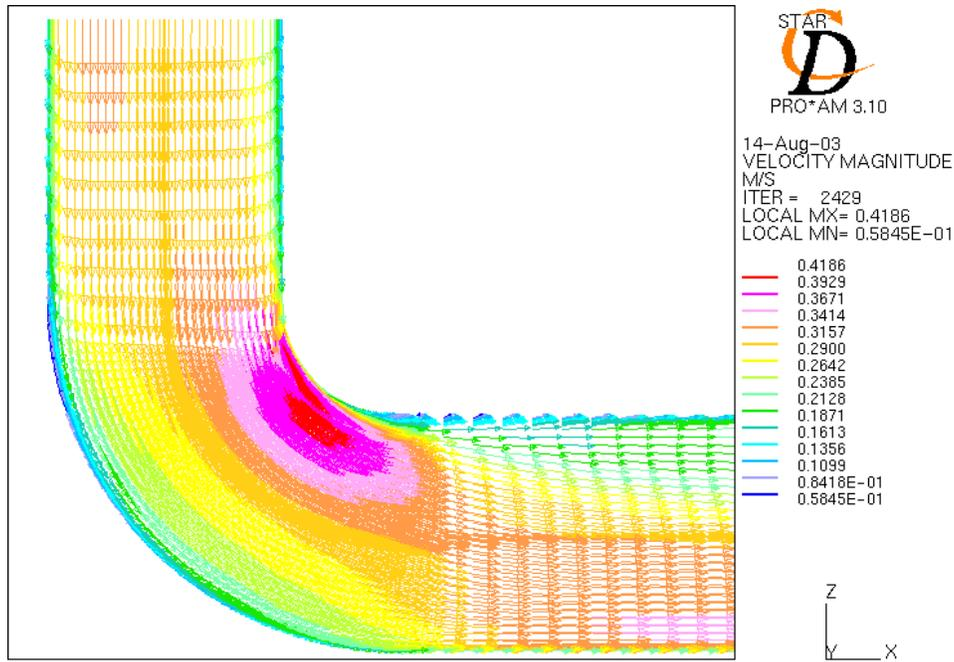
Figure 16: Velocity profile at an elbow section for the turbulent flow in the rectangular loop model
