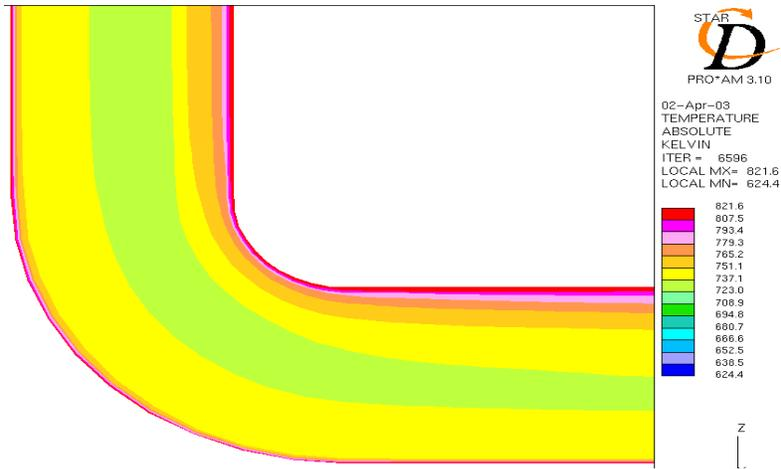
Figure 18: Temperature distribution for the turbulent flow in the rectangular loop model
