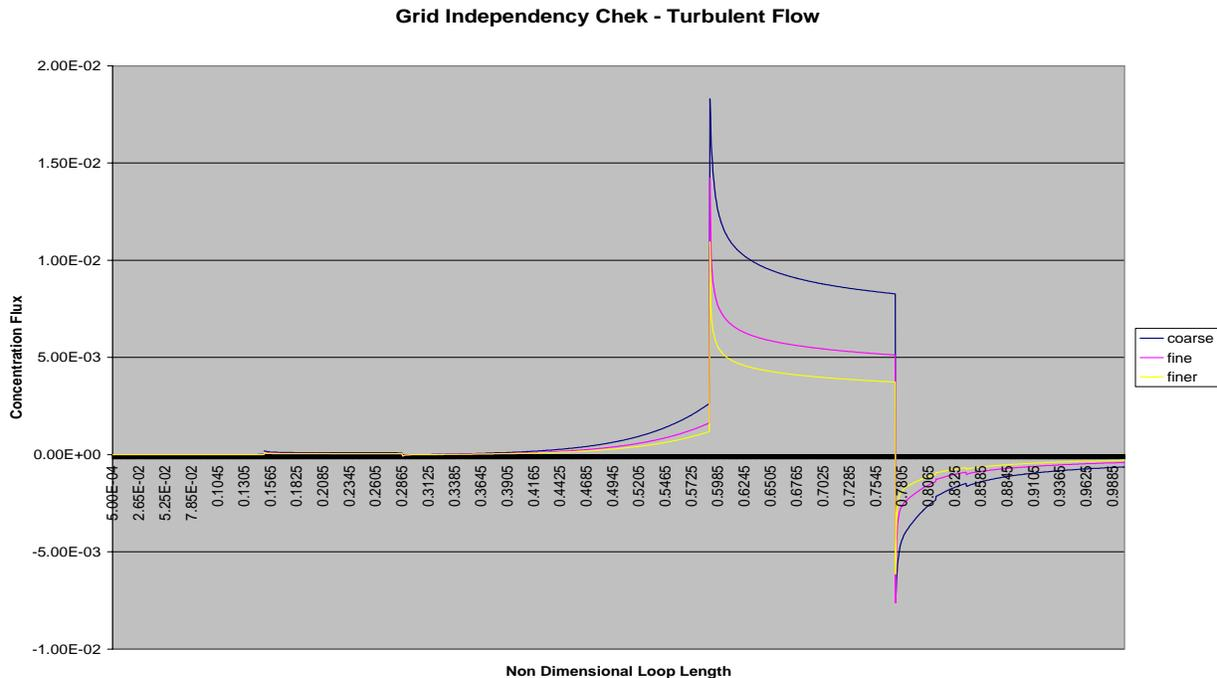
Figure – 8: Corrosion / Precipitation rate and Grid Independency Check for a Straight pipe model
