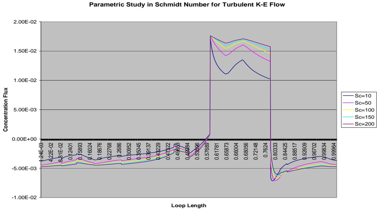
Figure – 26: Parametric Study in Schmidt Number for Turbulent Flow
