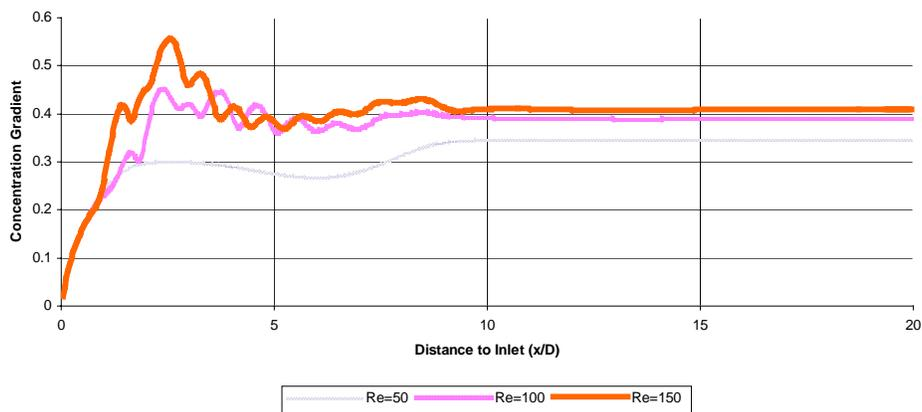
Figure – 35: Concentration gradient vs. distance to inlet at expansion ratio of 3
