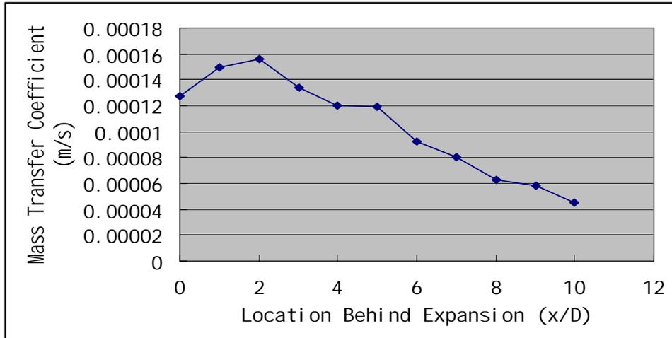
Figure – 45: Mass transfer coefficient variation at Re=1,000
