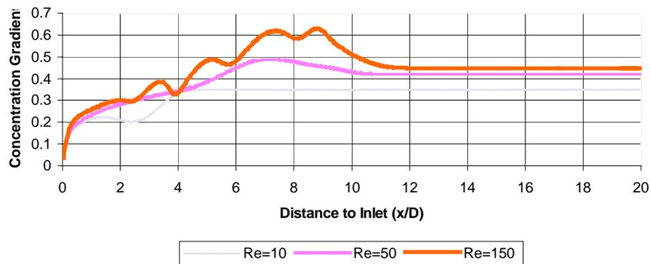
Figure – 33: Concentration gradient vs. distance to inlet at expansion ratio of 10
