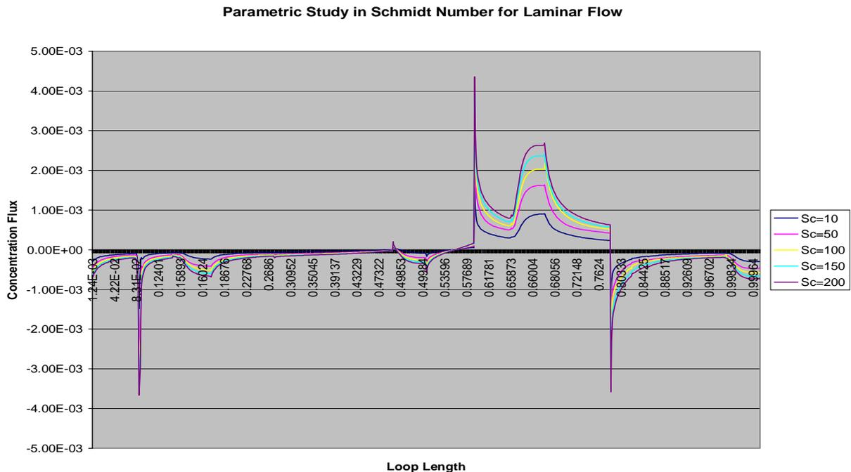
Figure – 25: Parametric study in Schmidt Number for Laminar Flow
