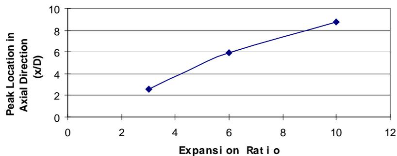
Figure – 36: Peak locations in axial direction for different expansion ratios
