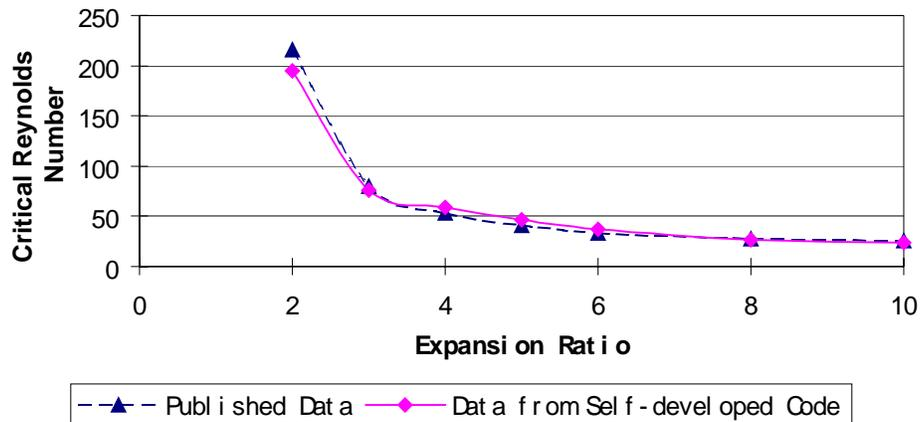
Figure – 32: Comparison of expansion ratios vs. critical Reynolds numbers between current study and Drikakis
