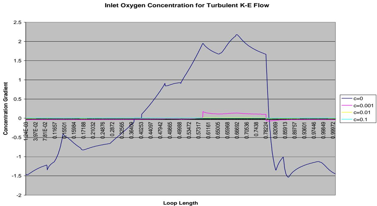
Figure – 28: Parametric Study in Initial Oxygen Concentration for Turbulent Flow
