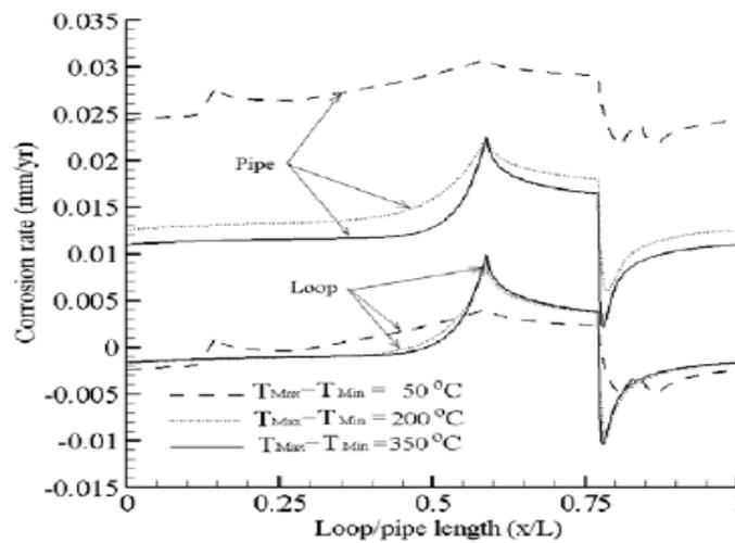
Figure – 7: Corrosion/precipitation rate from the analytical models
