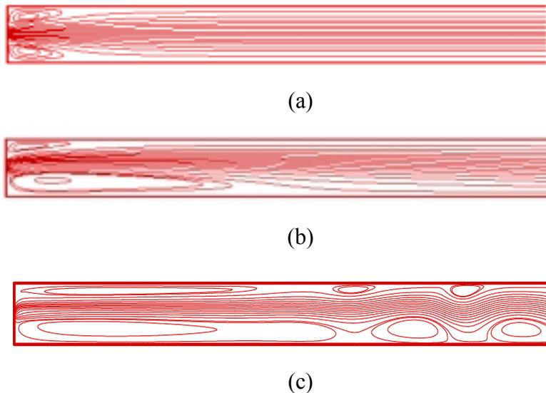
Figure – 31: Streamlines for Reynolds numbers equal to (a) 10, (b) 30 and (c) 150
