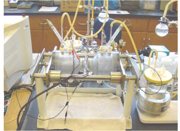
Figure 10. Devnathan-Staruchi cell schematic (left). Figure 11 Photograph of the actual hydrogen permeation cell [ASTM G148].
