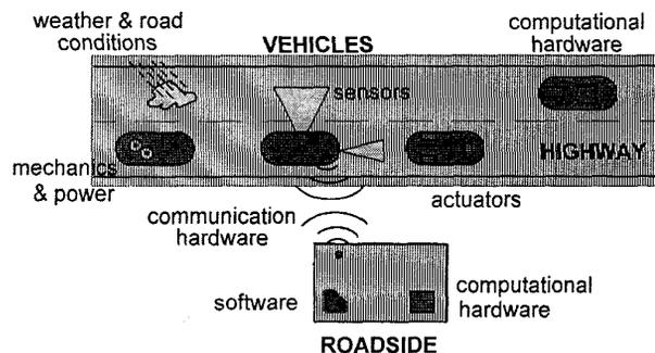
Figure 3. Sub-Systems of the FLASH Laboratory
