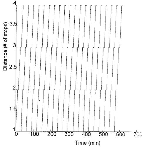
Fig. 5 Dynamics of bus behavior at steady state
