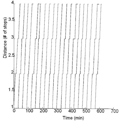
Fig. 6 Dynamics of bus behavior at nonsteady state
