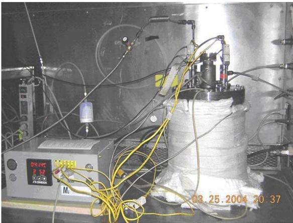
*Experimental apparatus developed in UNLV for the testing of the YSZ oxygen sensors.*
