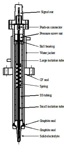
*Schematic of a YSZ Bi/Bi<sub>2</sub>O<sub>3</sub> oxygen sensor in a heating chamber. The reference solution of Bi/Bi<sub>2</sub>O<sub>3</sub> is filled and sealed inside the sensor core.*
