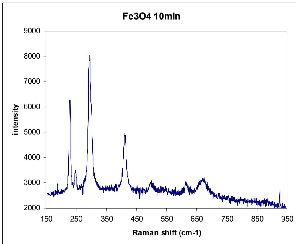
Figure 4. Note the new peak at 670 cm<sup>-1</sup>. The other peaks are Fe<sub>2</sub>O<sub>3</sub> peaks from impurities in the Fe<sub>3</sub>O<sub>4</sub> standard.
