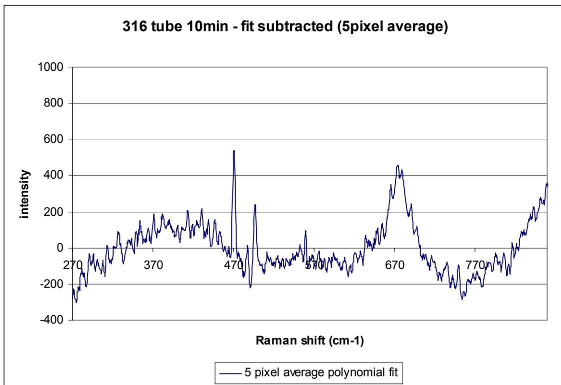
Figure 4. Annealed 316L exposed to LBE – 10 minute Raman spectra. Notice the peak at 670 cm<sup>-1</sup>, characteristic of Fe<sub>3</sub>O<sub>4</sub>.
