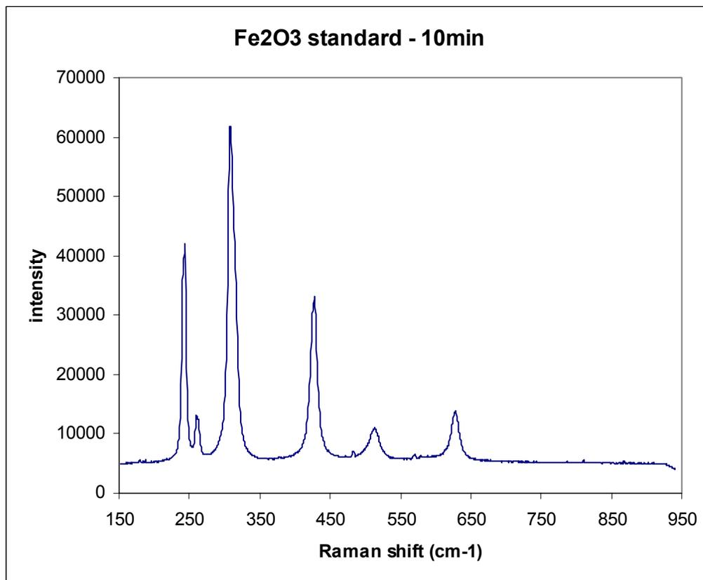
Figure 3. Raman spectrum of  $\text{Fe}_2\text{O}_3$  standard.
