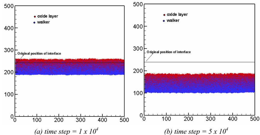
*Snapshots of the simulated layer in the presence of corrosion with scale removal. They correspond to  $2.5 \times 10^4$  time step. The red dot is the oxide site; The blue dot is the walker site; The upper side of the layer is filled with solvent; The lower side of the oxide layer is pure metal. The corrosion probability of metal is taken as 0.5. The possibility of scale removal of the oxide site close to solvent is 0.004.*
