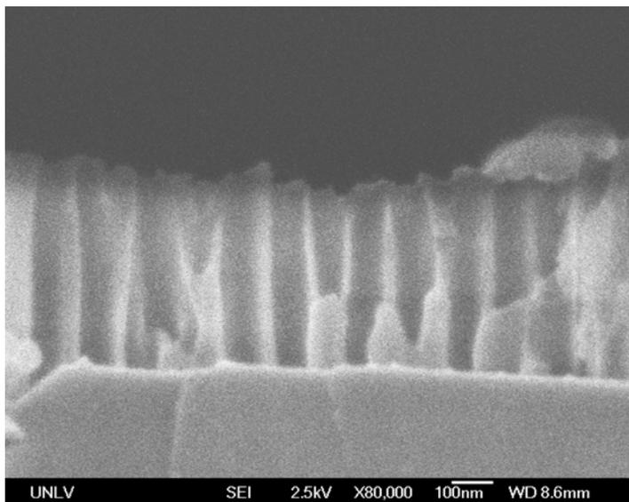
Cross-sectional FESEM image of Cr nanowires inside a porous alumina template showing non-uniform distribution of nanowires.
