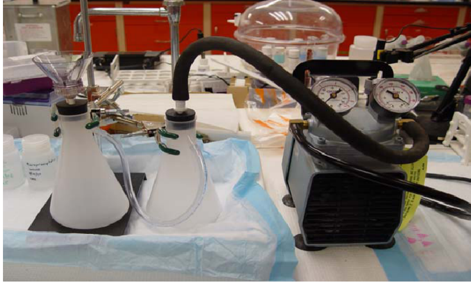
Figure 2.1 Single Filtration Setup (Stock 2007)
