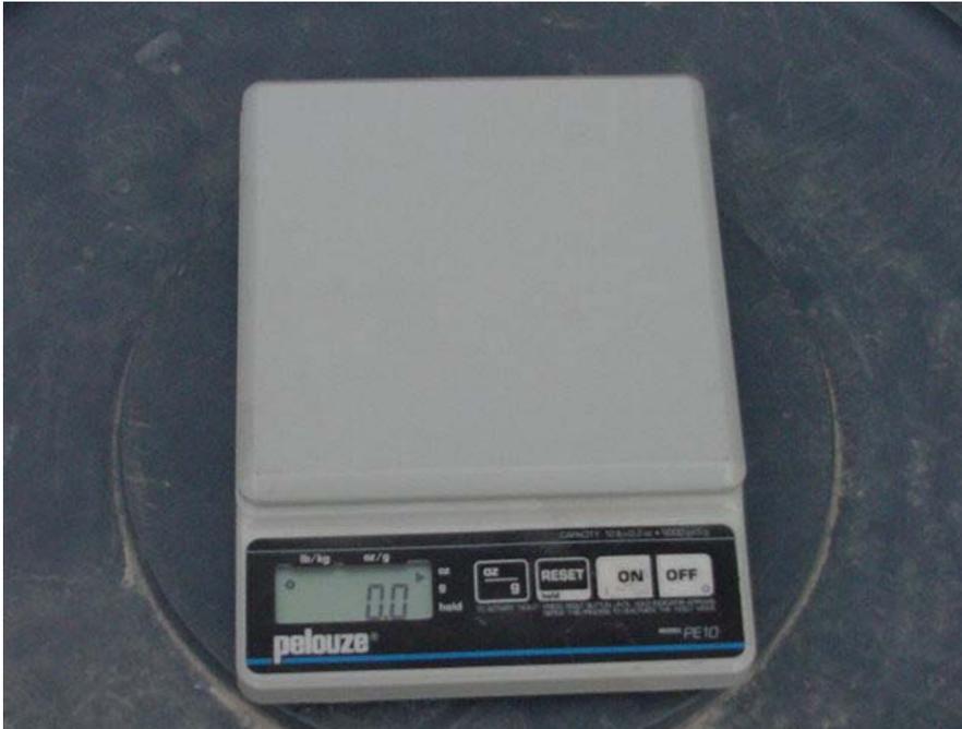
A 7 quart trash container was used for weighing recyclables and a 13 quart container was used for the trash as seen in Figure 4 and 5. By placing the bin on the scale and pressing the “reset” button so the scale would be tared, or would read zero. Then the recyclables were put in and weighed. Weighing was conducted in a covered area to prevent wind error.
