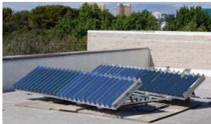
FIGURE 1. Photograph shows JXC carousel tracker with four 3-sun mirror modules in operation and under test at UNLV since 2008.
